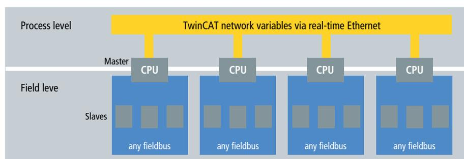
Fig. 4 Different communication channels at the field and process level
