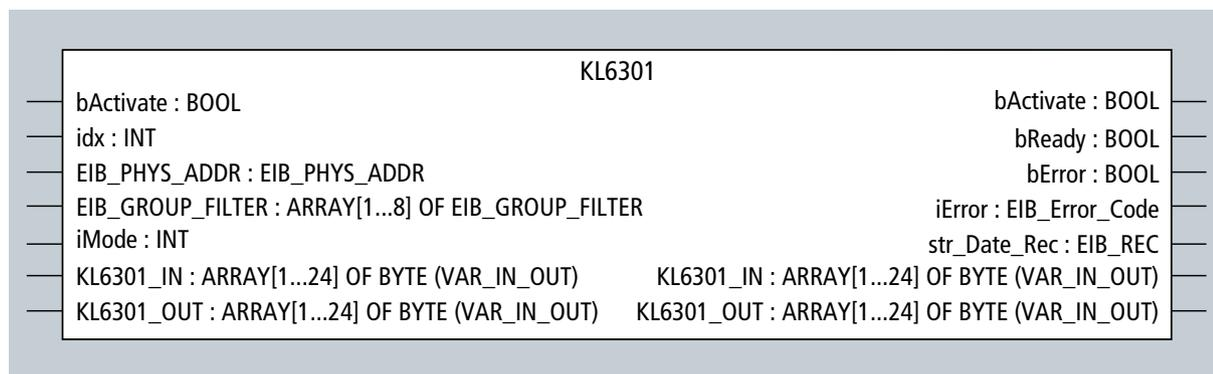
Fig 5 FB\_KL6301 for communication of the EIB terminal with the devices
