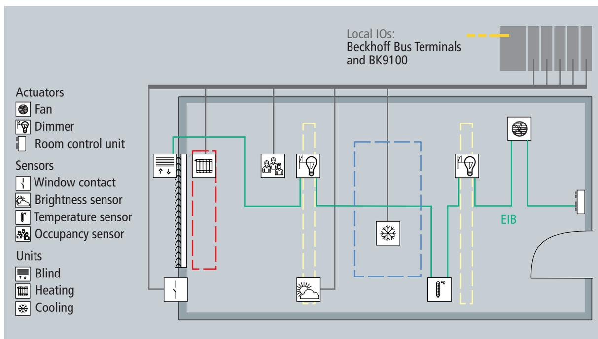
Fig. 8 Each office represents a unit, which can be controlled separately via an EIB room control unit.
