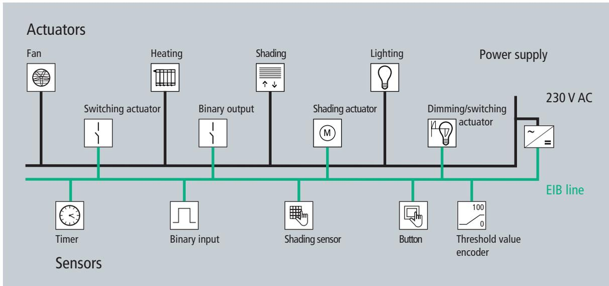
Fig.3 Separation of supply voltage and control voltage
