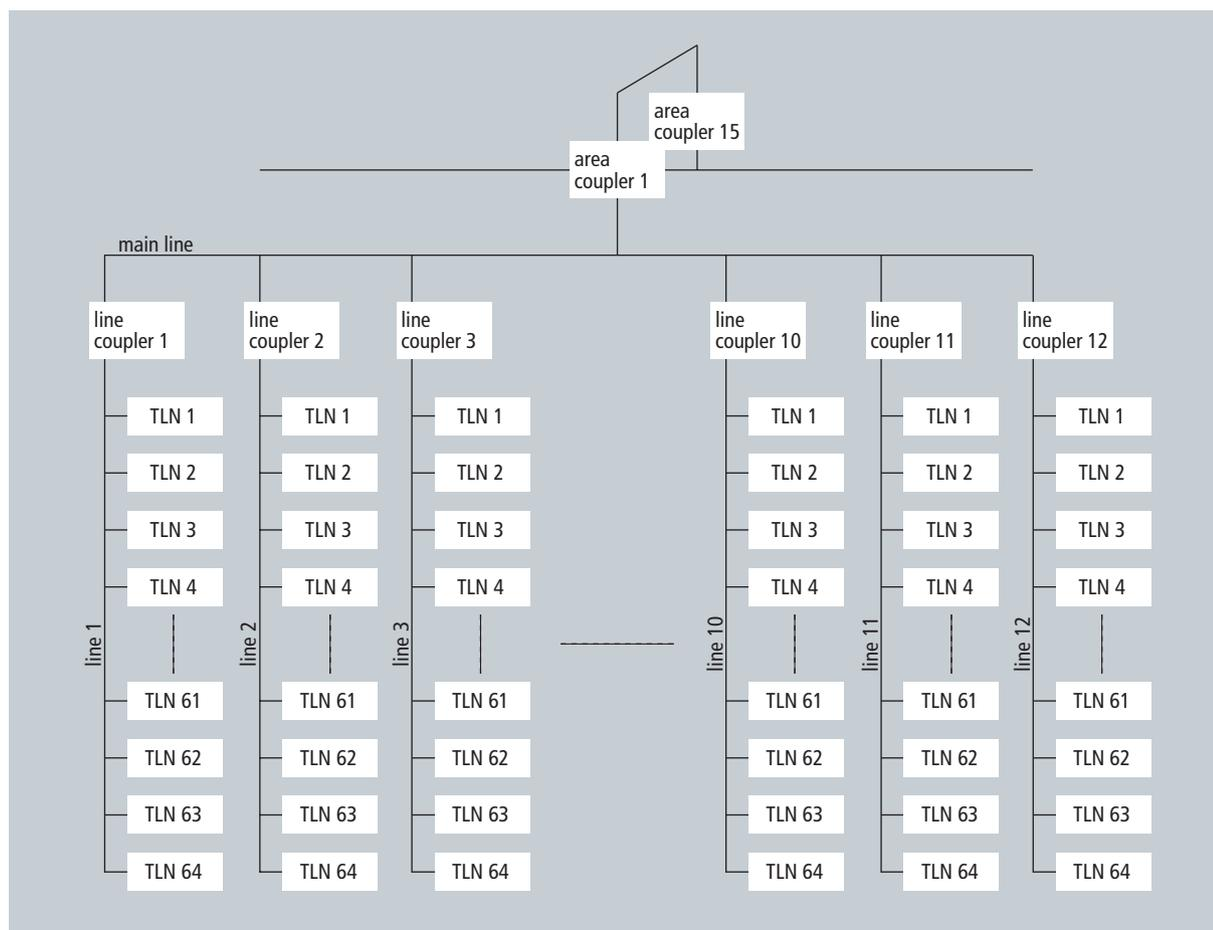
Fig. 1 Grouping of EIB devices in lines, main lines and area lines
