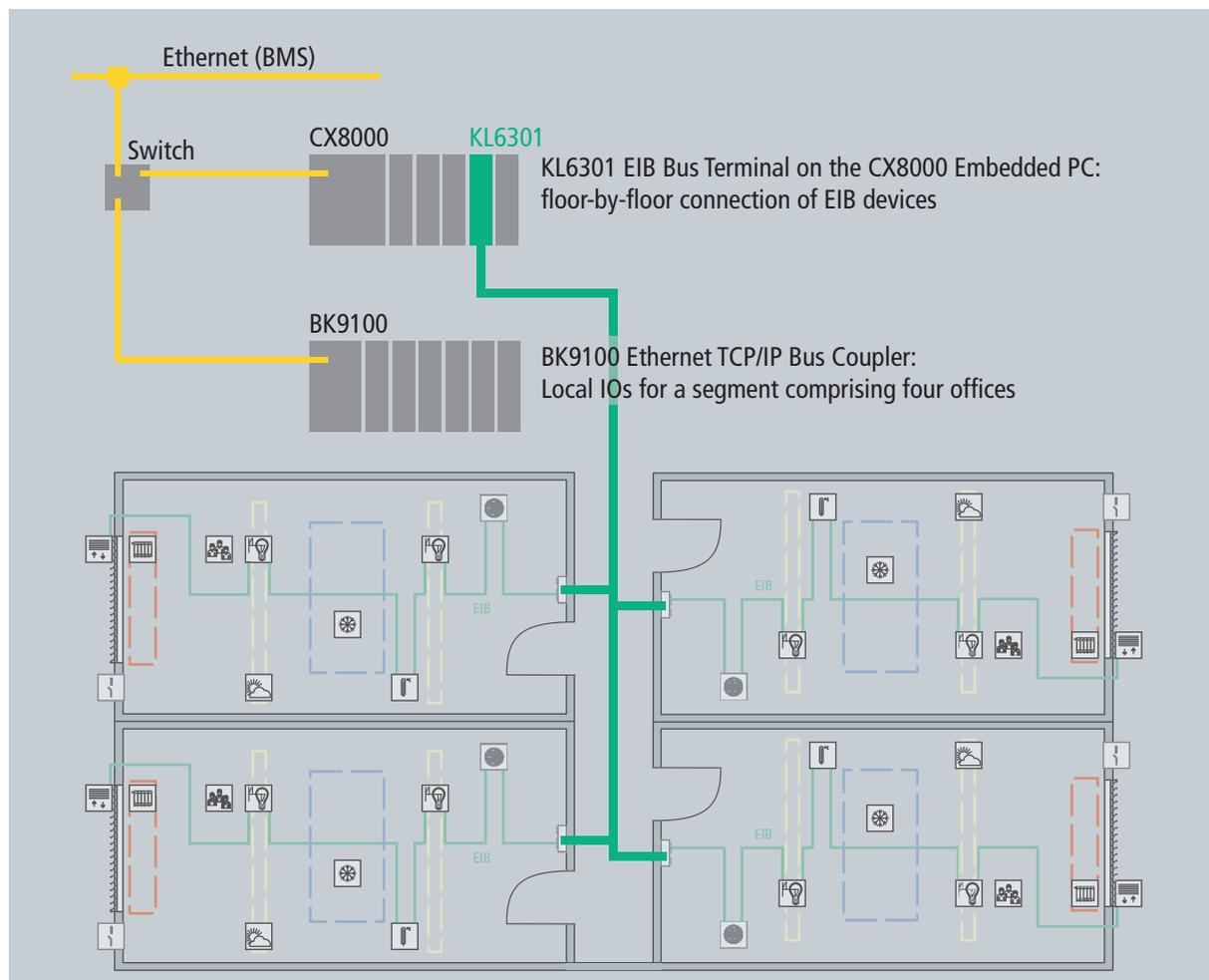
Fig. 9 Bundling of the offices on a floor via EIB and grouping of the devices within the controller according to trades
