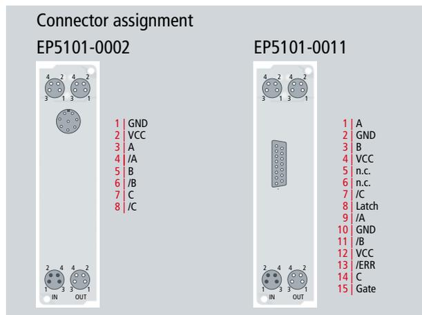
Fig. 4 Connector assignment of the EP5101 EtherCAT Box
