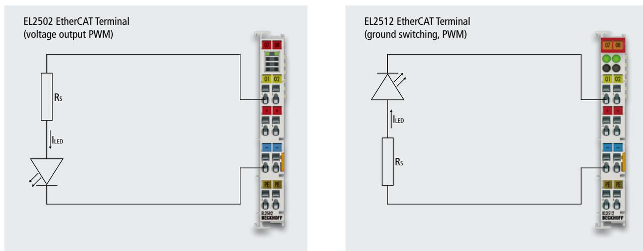
Figure 5: Monochrome LED at a pulsating output
