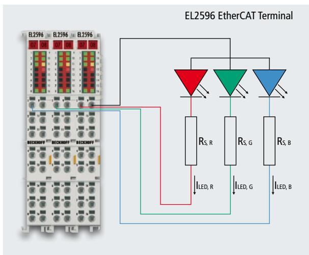
Figure 4: Multicolored LEDs with EL2596 LED control source
