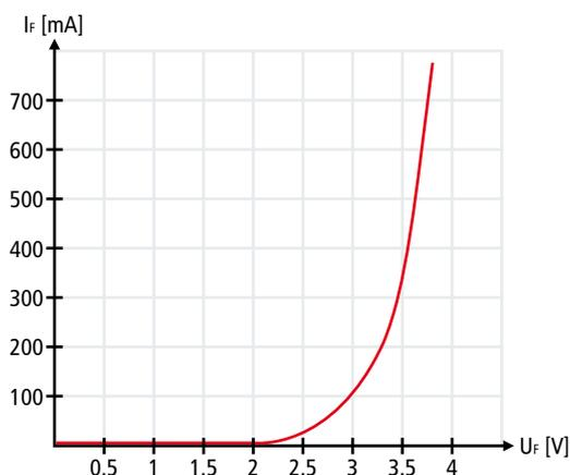
Figure 1: Example characteristic curve of an LED
