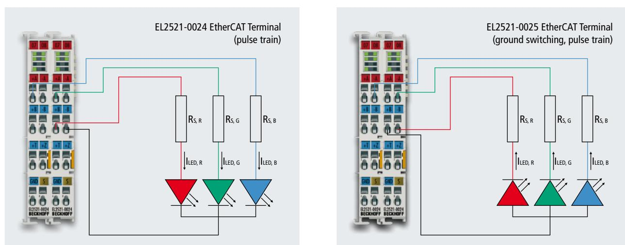
Figure 8: Multicolored LED at a pulsating output
