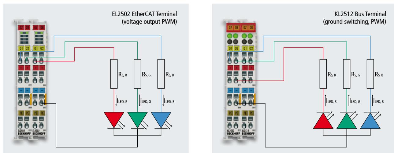
Figure 6: Multicolored LED at a pulsating output
