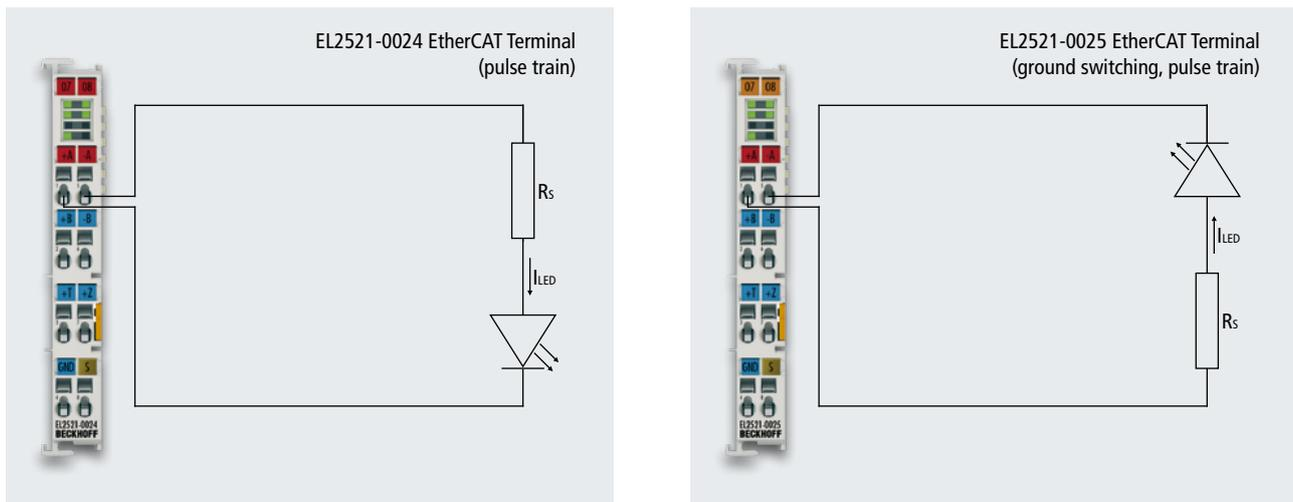
Figure 7: Monochrome LED at a pulsating output
