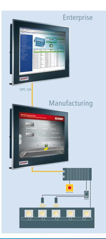
"SAP Manufacturing Execution demo" from SAP and Beckhoff is a real industry solution to demonstrate the connection between the Beckhoff PLC controllers in the manufacturing and the SAP enterprise world. In a perfect plant, the information on all processes is seamlessly integrated and consistent. This enables you to make the right business decisions in a timely fashion.
