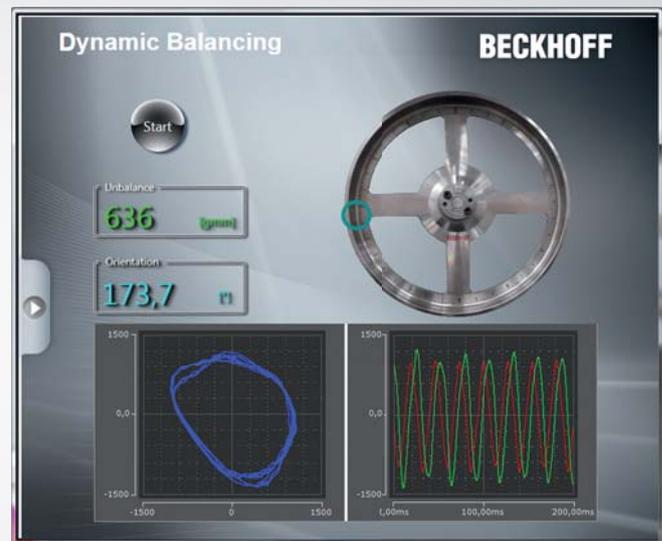
Fig. 5: Two Scope controls integrated in a .NET application
