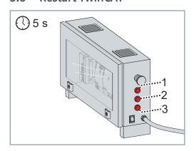
► Press the Start button [1], Stop button [2], and Reset button [3] simultaneously for 5 seconds to restart TwinCAT
