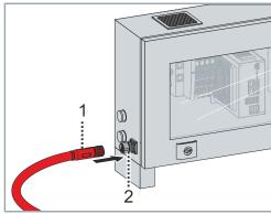
► Plug the connector [1] of the connection cable into the connector [2] of the control cabinet
