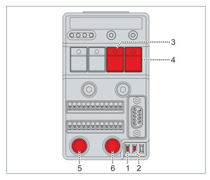
The position of the switches [1] and [2] on the test board determines whether the digital inputs [3] and [4] or the analog inputs [5] and [6] are enabled.
