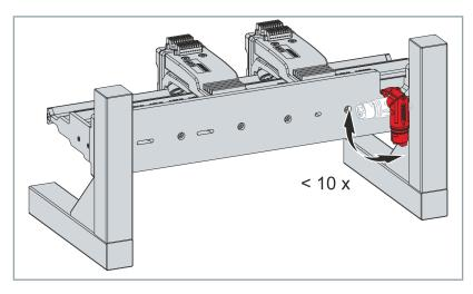
The connector of the module may be rotated by 90° a maximum of ten times.
