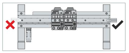
The rail on support may only be mounted on the motor module without connectors.
