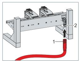
▶ Plug the connector [1] of the connection cable to the connector [2] of the module
