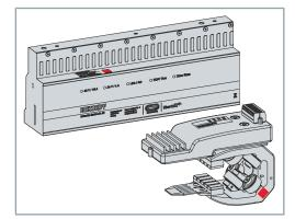
The DataMatrix code can be found on all movers and modules. If there is no Beckhoff Traceability Number (BTN) under the DataMatrix code, you can read it out via the DataMatrix code.
