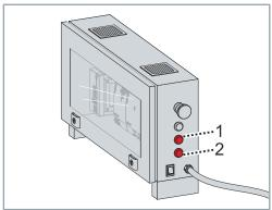
The *Stop* button [1] must light up red continuously. The *Reset* button [2] must flash blue.
