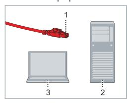
▶ Plug the connector [1] of the data line into the corresponding port of your PC [2] or laptop [3]
