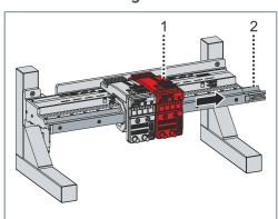
► Remove the mover [1] via the rail on support [2]
