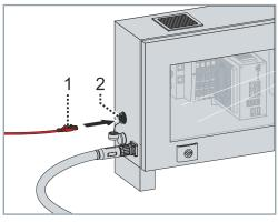
► Connect the connector [1] of the data line to the connector [2] in the control cabinet
