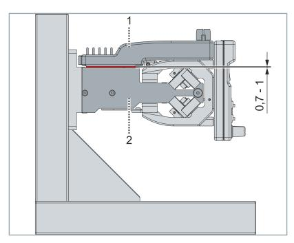
The air gap between the mounted NCT electronics [1] and the motor module [2] is preset to 1 mm ex factory. The air gap may be reduced to a minimum of 0.7 mm.
