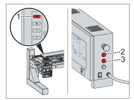
The Power LED [1] on the NCT electronics light up continuously.
