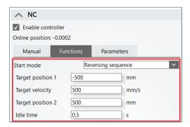
With the "Reversing sequence" function, you can move your axes between a defined start position and the end position.
