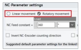
In the selection area for "NC parameter settings" you can size your mechanical system and thus determine the "NC Feed constant".
