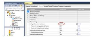
Following-error monitoring should be disabled for the NC axis or set to a large value so that it is not triggered in the following tests.
