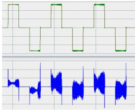
Depending on the mechanical system, the value that was reached can be regarded as Kp<sub>crit</sub>, or Kp can be increased further, until the oscillation also shows up in the velocity value. It will then also be more audible.
