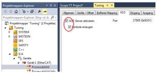
In the process image of the EtherCAT master activate the ADS server and the symbol generation facility.
