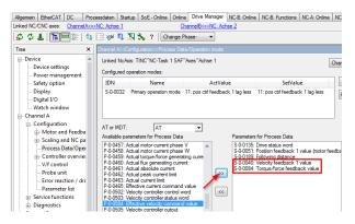
The axes are then shown one below the other. Add the "Torque feedback value" (S-0-0084), the velocity command value and the actual velocity value (P-0-0504 and S-0-0040) to the AX5000 process data.
