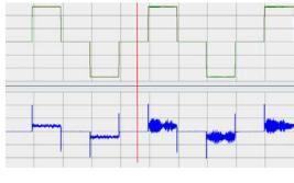
While the axis reverses, observe the behavior with the oscilloscope. The following oscilloscope pattern shows the velocity command value and actual velocity value in the upper diagram and the current or torque ("torque feedback value") in the lower diagram.
