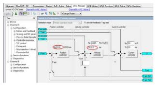
In most cases the AX5000 operates in mode "11: Position control feedback 1". In order to eliminate the influence of the position controller, Kv should be 0 for the tuning process in the position controller. In addition, Tn is set to 0 in the velocity controller.
