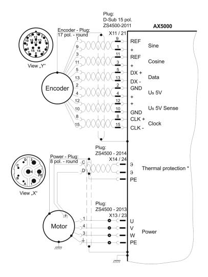
\* If no ConnectorBox is used, the ZK4540-0020-xxxx thermal protection contact cable is additionally required. This is to be connected to X14 / 24.
