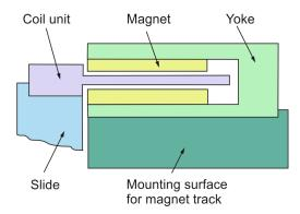
The mounting surfaces for the magnet yokes and the coil unit must be extremely even, in order to prevent bending forces.
