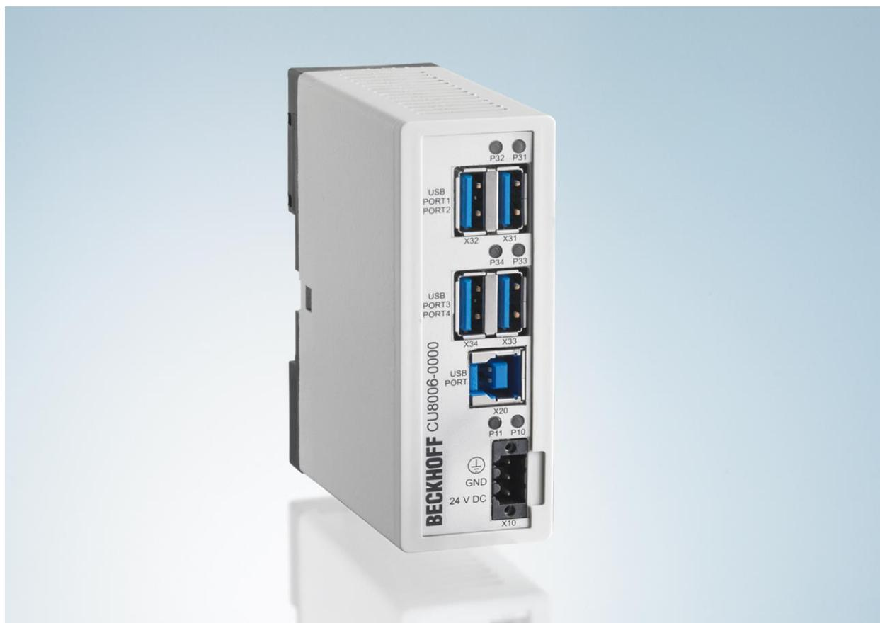
The CU8006 DIN rail-mount USB hub has four ports and supports the USB 3.0 data transfer rate of up to 5 Gbit/s, but is also compatible with slower USB standards. USB 3.0 devices can be connected at a distance of up to 3 m. Connection to USB 1.1/ USB 2.0 devices is possible with 5-m cables.
