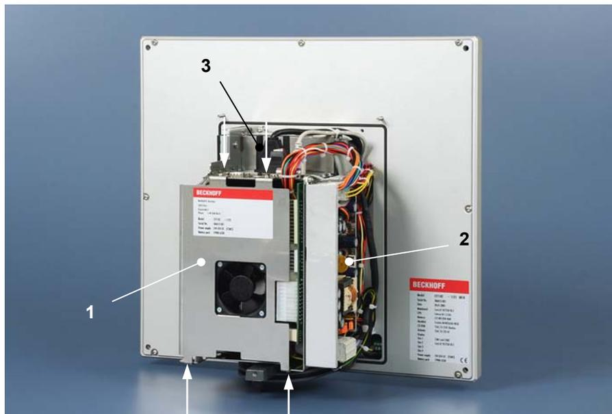
Removing the outer housing provides access to the inner chassis (1), the power supply unit (2) and the interfaces (3) of the PC. The inner chassis is fastened with 4 crosshead screws (see arrows).
