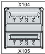
Fig. 6: CP69xx\_USB output pin numbering
