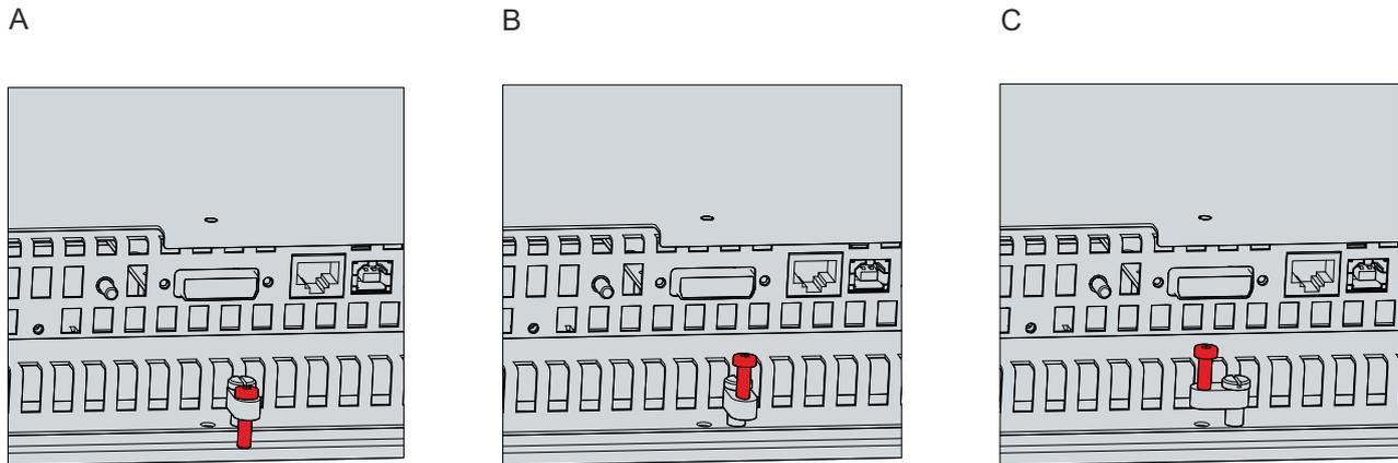
Fig. 16: CP69xx\_removal from the control cabinet
