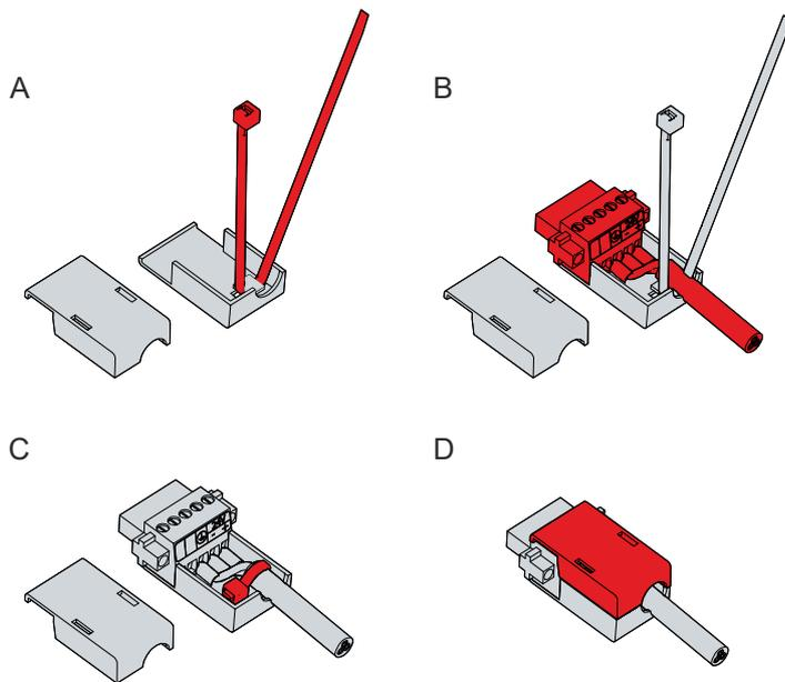
Fig. 13: CP69xx\_assembly of strain relief housing
