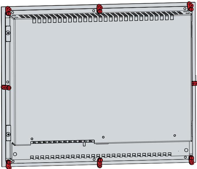
Fig. 10: CP69xx\_delivery state clamping lever
