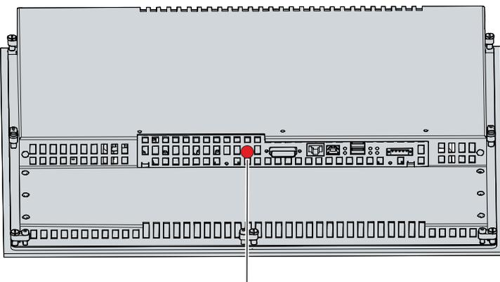
Fig. 15: CP69xx\_grounding bolt functional earthing
