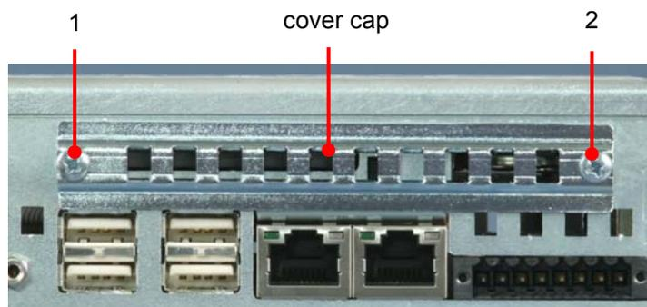
After solving the two crosshead screws (1) und (2), the cover cap can be removed and allows access to the CF-Card and the battery.
