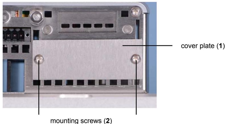
For mounting of a plug-in card first unloose the screws (2). The cover plate (1) can now be removed and allows to plug in the card.
