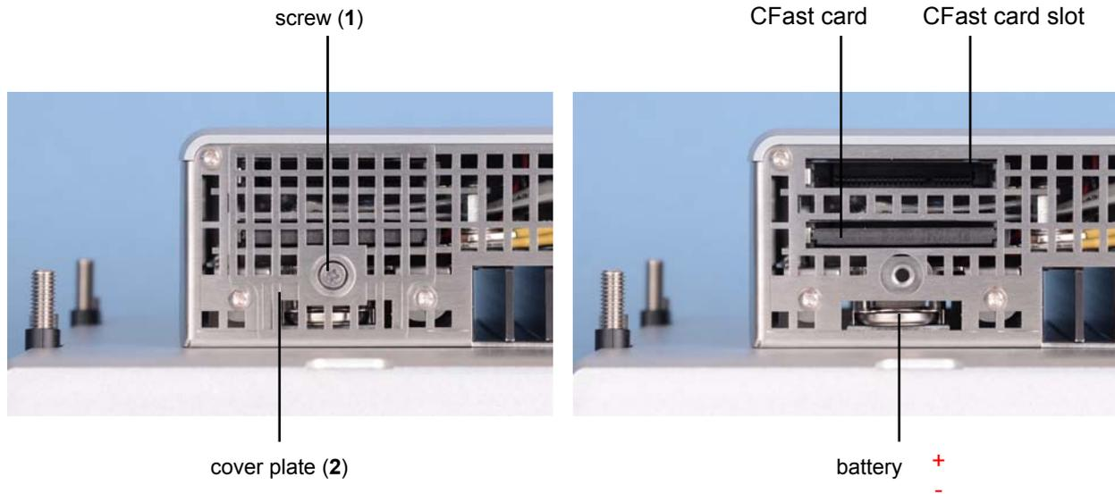
For replacing the battery and installation of the CFast cards first unloose the cross-head screw (1). The cover plate (2) can now be removed.
