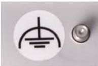
Earthing connections dissipate interference from external power supply cables, signal cables or cables to peripheral equipment.
