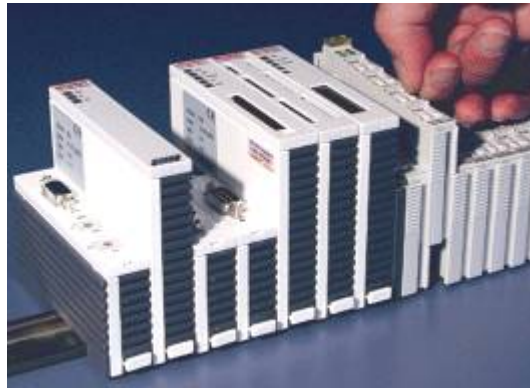
FIG. 2: Releasing the I/O terminal from the top-hat rail
