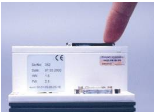
Figure 3 Inserting the CF card
