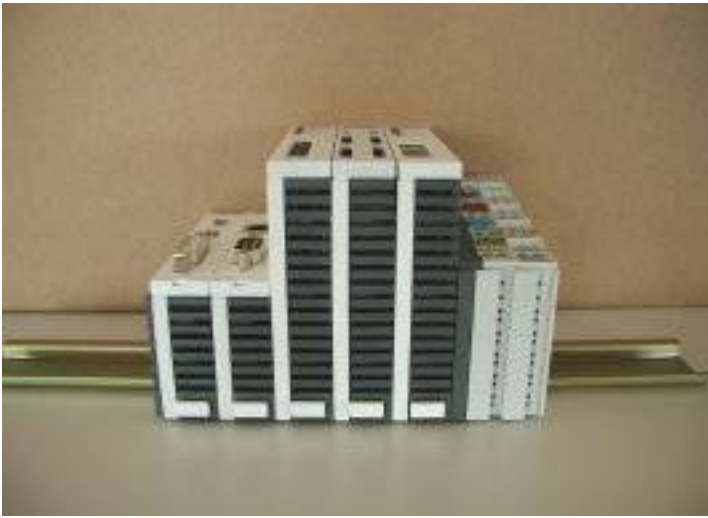
FIG. 9: Allowable installation position
