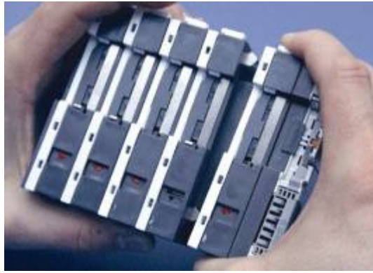
FIG 5: Separating the modules
