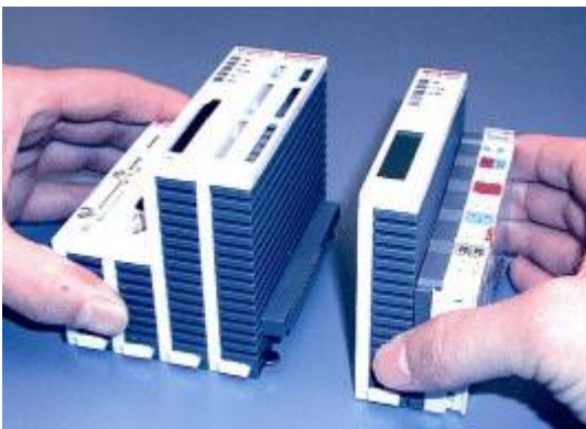
FIG. 1: Engaging of the Modules
