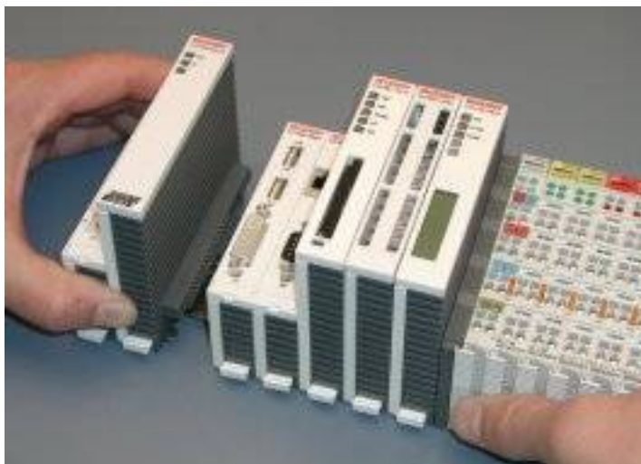
FIG. 3: Stick modules together
