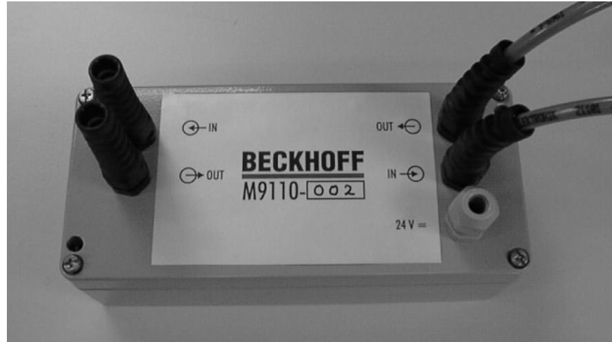
The bidirectional Beckhoff Lightbus amplifier M9110 is used for polymer fibre optic cable with a length of more than 45 m, and if glass fibre optic cable should not be used.
