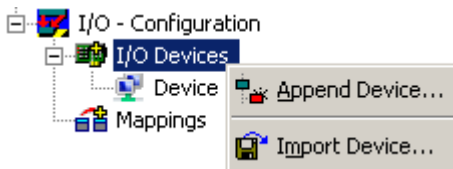
Fig. 50: Creating a new device
