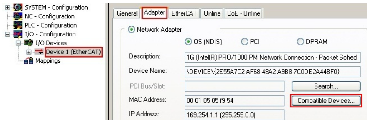
Fig. 33: EtherCAT device properties (TwinCAT 2): click on “Compatible Devices...” of tab “Adapter”
