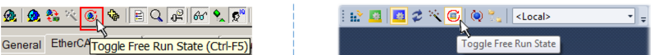
Fig. 68: TwinCAT can also be switched to this state by using a button (left: TwinCAT 2; right: TwinCAT 3)
