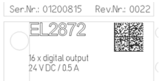
Fig. 1: EL2872 with revision 0022 and serial number 01200815
