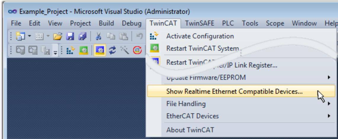
Abb. 61: Aufruf in VS Shell (TwinCAT 3)
