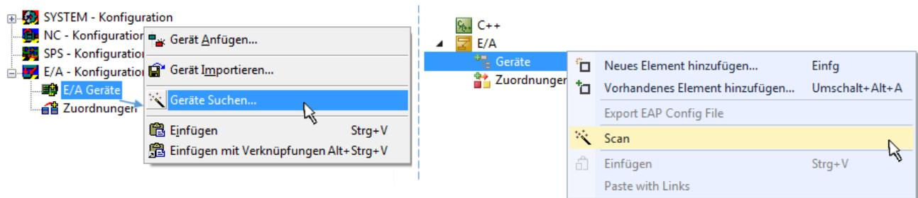
Abb. 88: Scan Devices (links: TwinCAT 2; rechts: TwinCAT 3)
