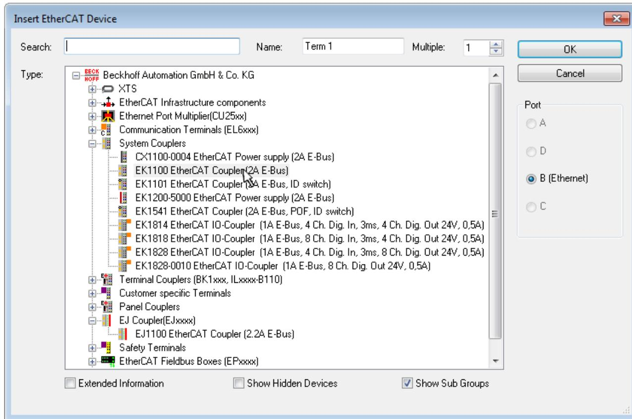
Fig. 79: Selection dialog for new EtherCAT device
