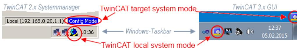
Fig. 84: Differentiation local/target system (left: TwinCAT 2; right: TwinCAT 3)
