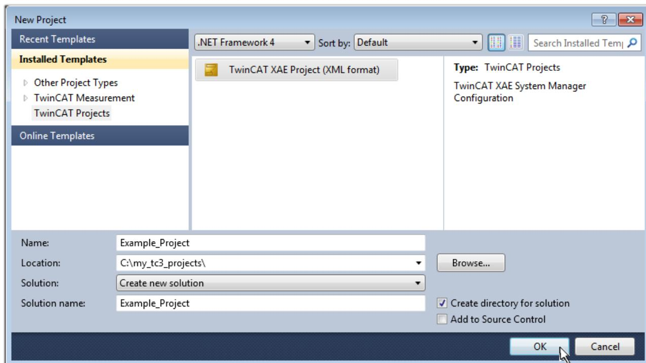
Fig. 37: Create new TwinCAT project
