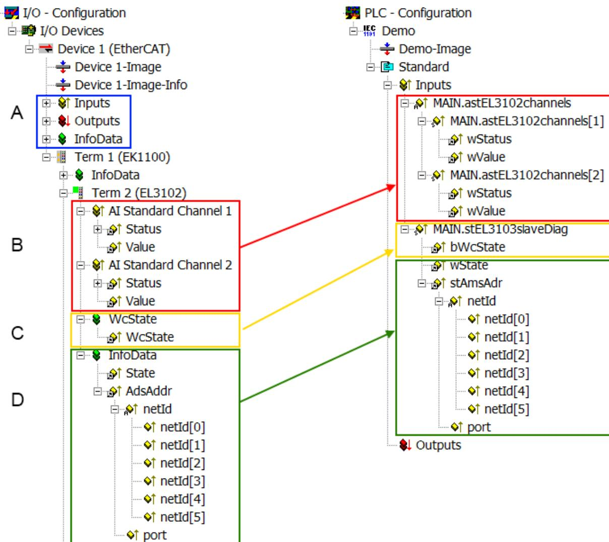
Fig. 116: Basic EtherCAT Slave Diagnosis in the PLC
