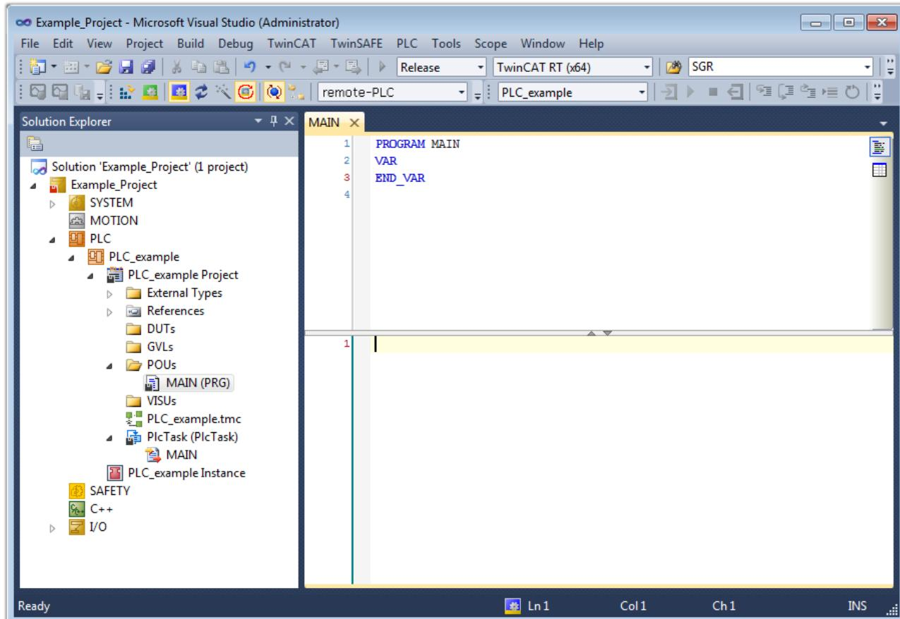
Fig. 47: Initial “Main” program of the standard PLC project
