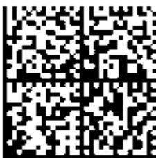
Fig. 3: Example DMC **1P**072222**SBTN**k4p562d7**1K**EL1809 **Q**1 **51S**678294
