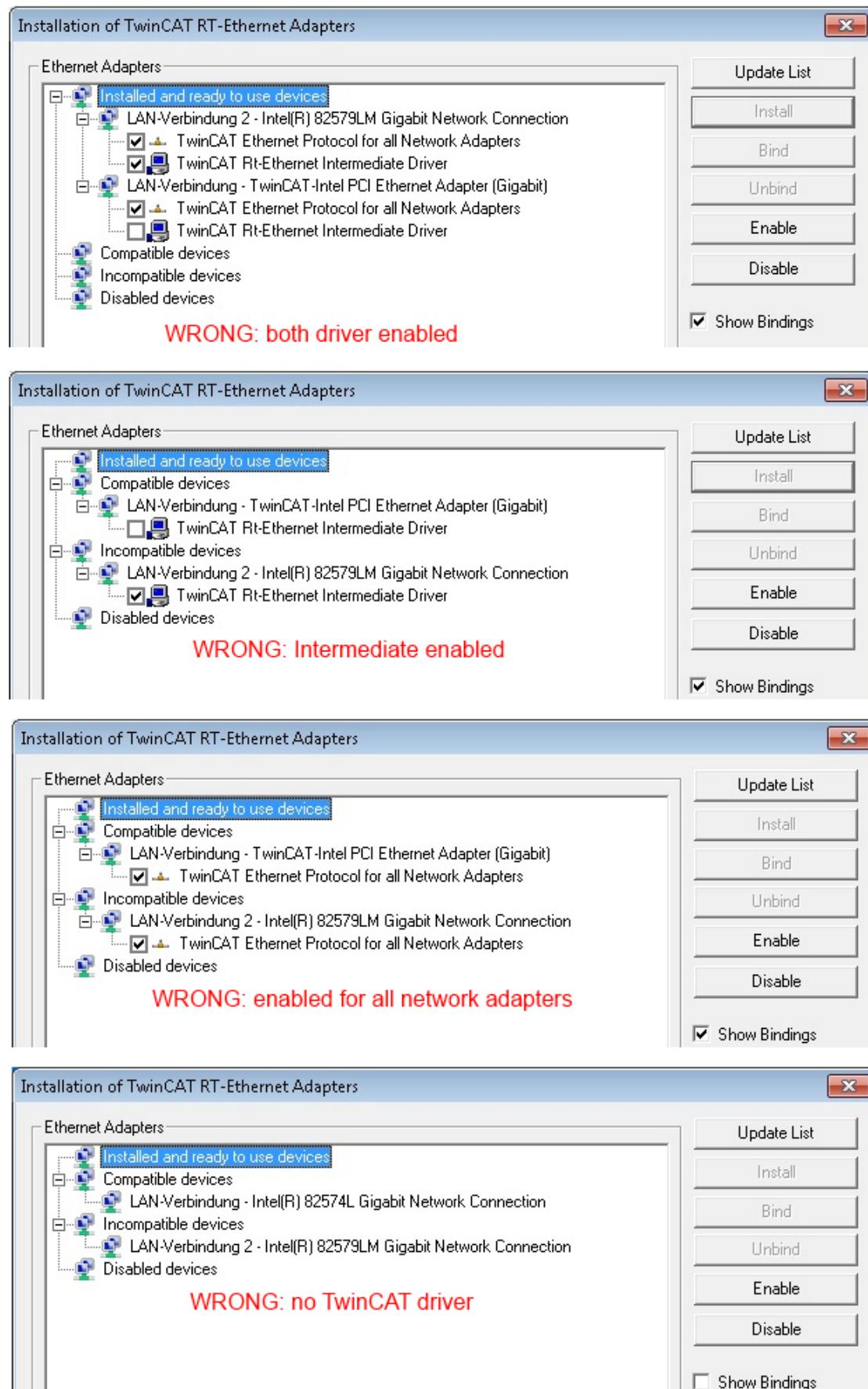
Fig. 66: Incorrect driver settings for the Ethernet port
