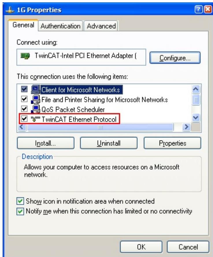
Fig. 64: Windows properties of the network interface
