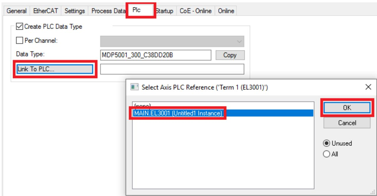
Fig. 56: Linking the structure
