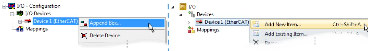
Fig. 78: Appending EtherCAT devices (left: TwinCAT 2; right: TwinCAT 3)
