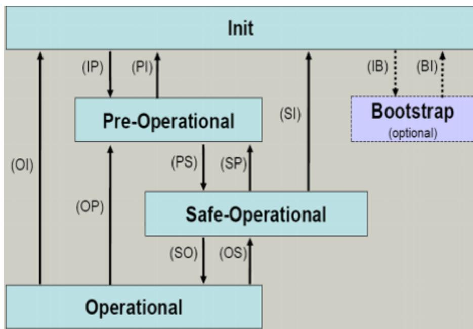
Fig. 7: States of the EtherCAT State Machine
