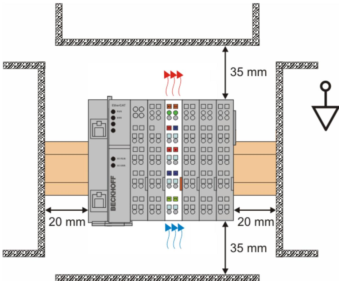
Fig. 13: Recommended distances for standard installation position
