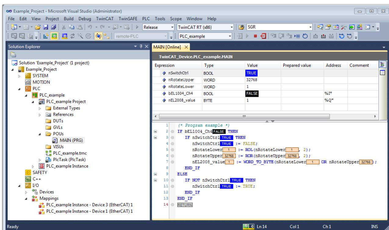
Fig. 58: TwinCAT development environment (VS shell): logged-in, after program startup
