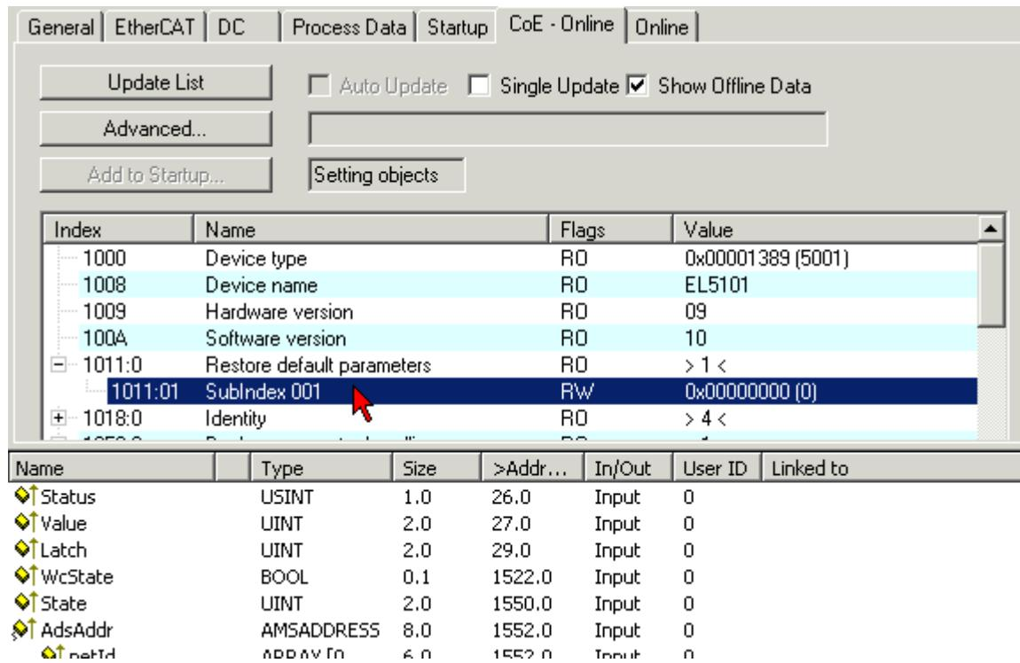
Fig. 145: Selecting the *Restore default parameters* PDO
