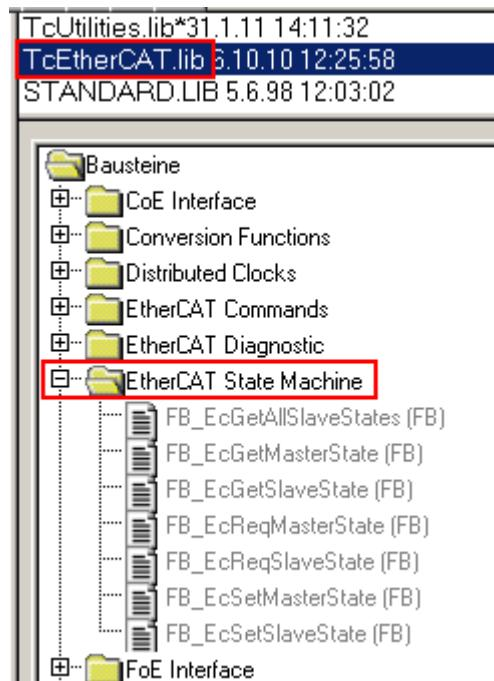
Fig. 121: PLC function blocks
