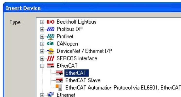
Fig. 75: Selecting the EtherCAT connection (TwinCAT 2.11, TwinCAT 3)
