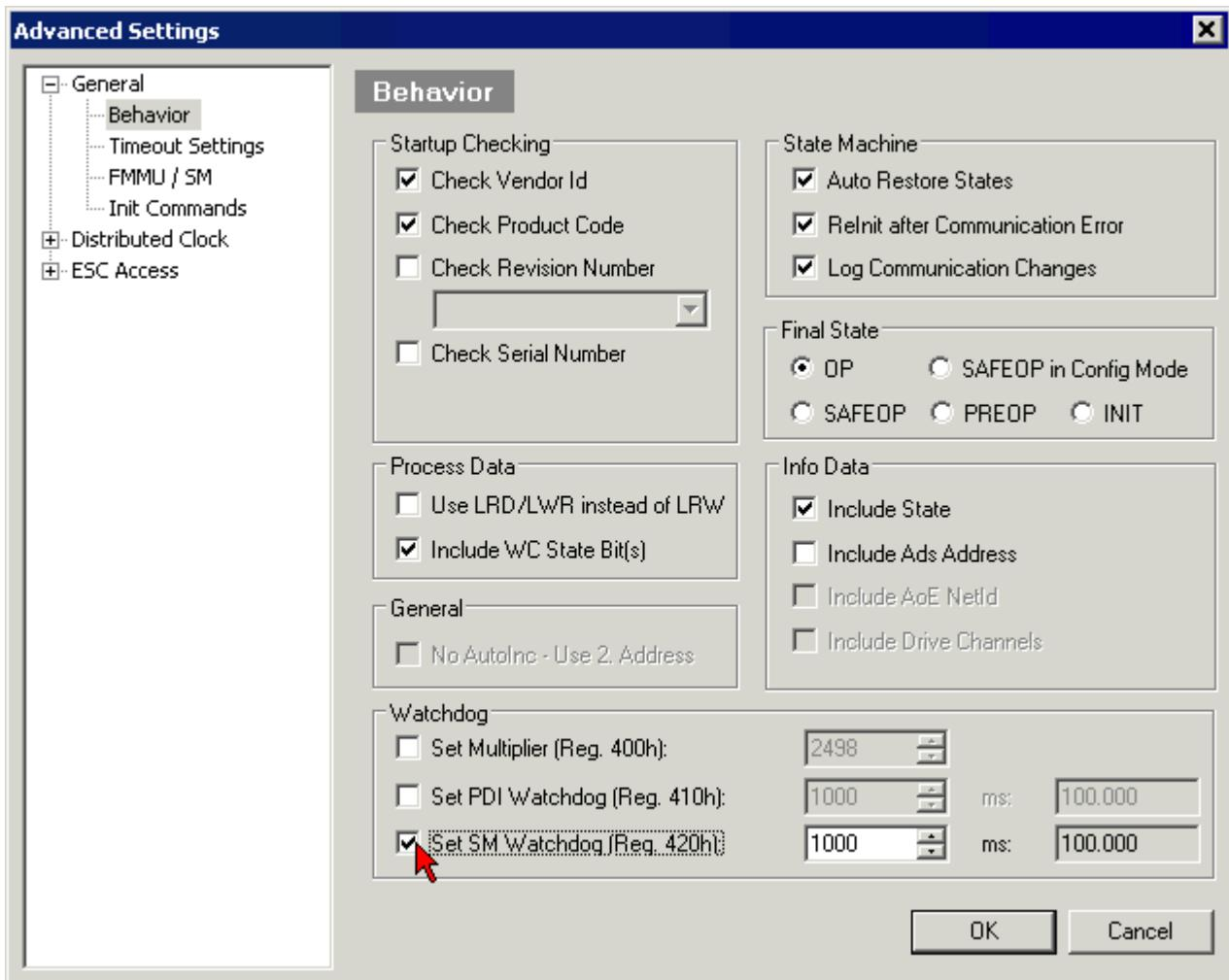
Fig. 6: EtherCAT tab -> Advanced Settings -> Behavior -> Watchdog
