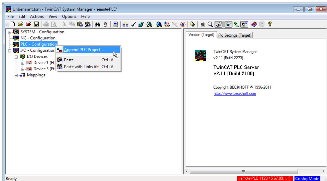
Fig. 28: Appending the TwinCAT PLC Control project
