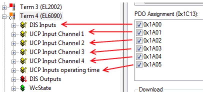
Fig. 124: Assignment of the inputs to the PDOs
