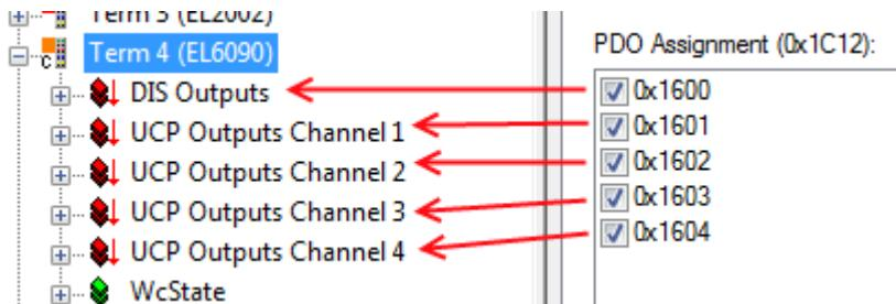
Fig. 125: Assignment of the outputs to the PDOs
