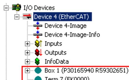
Fig. 98: Faulty identification
