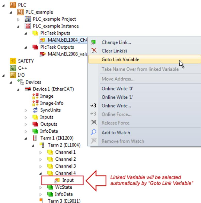
Fig. 53: Application of a “Goto Link” variable, using “MAIN.bEL1004\_Ch4” as a sample
