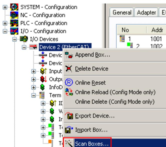
Fig. 134: Scan the subordinate field by right-clicking on the EtherCAT device
