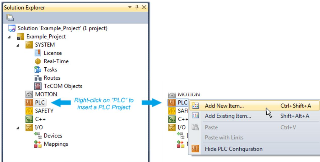
Fig. 45: Adding the programming environment in “PLC”
