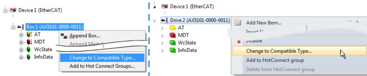
Fig. 103: Dialog "Change to Compatible Type..." (left: TwinCAT 2; right: TwinCAT 3)
