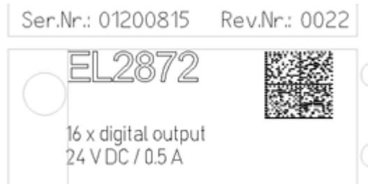
Fig. 1: EL2872 with revision 0022 and serial number 01200815
