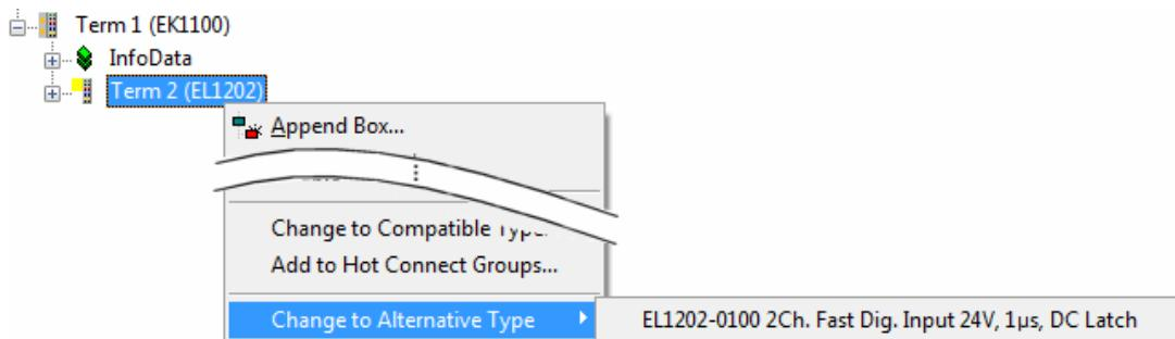
Fig. 104: TwinCAT 2 Dialog Change to Alternative Type
