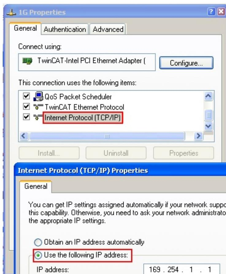
Fig. 67: TCP/IP setting for the Ethernet port
