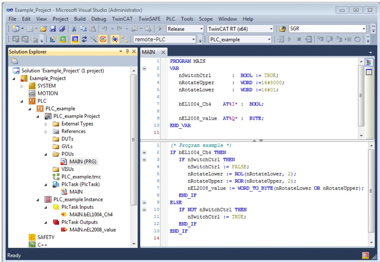
Fig. 48: Sample program with variables after a compile process (without variable integration)
