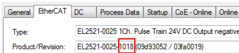
Fig. 89: Installing EtherCAT terminal with revision -1018
