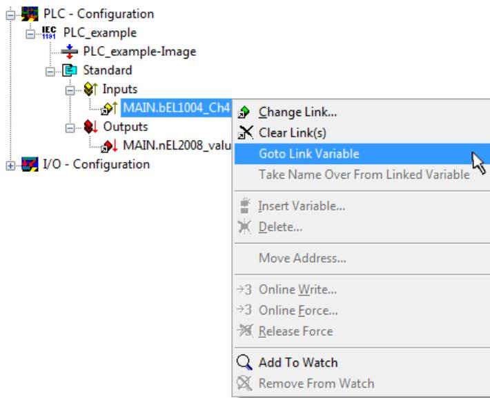
Fig. 33: Application of a “Goto Link” variable, using “MAIN.bEL1004\_Ch4” as a sample
