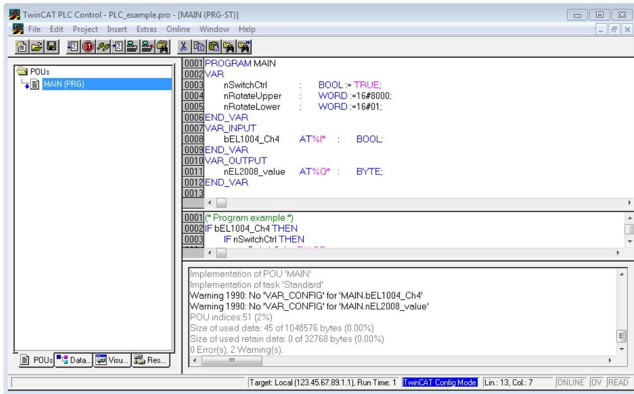
Fig. 27: Sample program with variables after a compile process (without variable integration)
