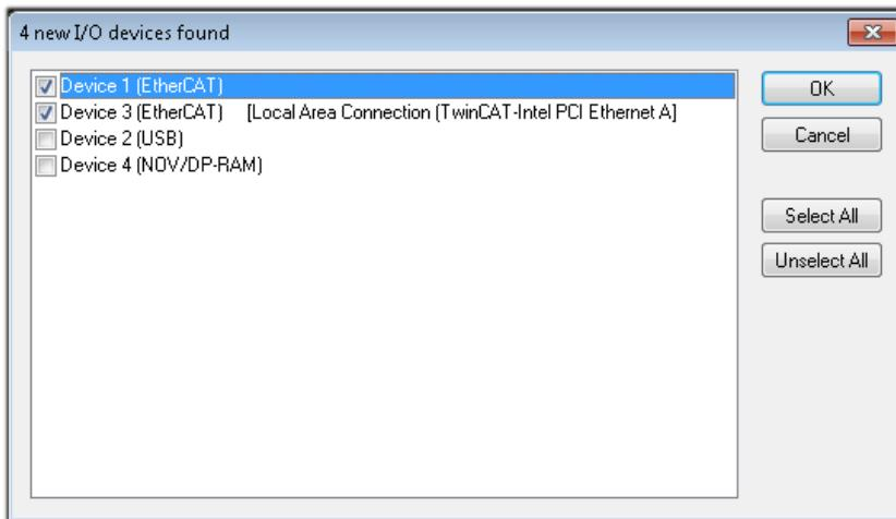
Fig. 23: Automatic detection of I/O devices: selection the devices to be integrated
