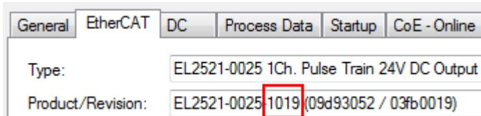
Fig. 90: Detection of EtherCAT terminal with revision -1019
