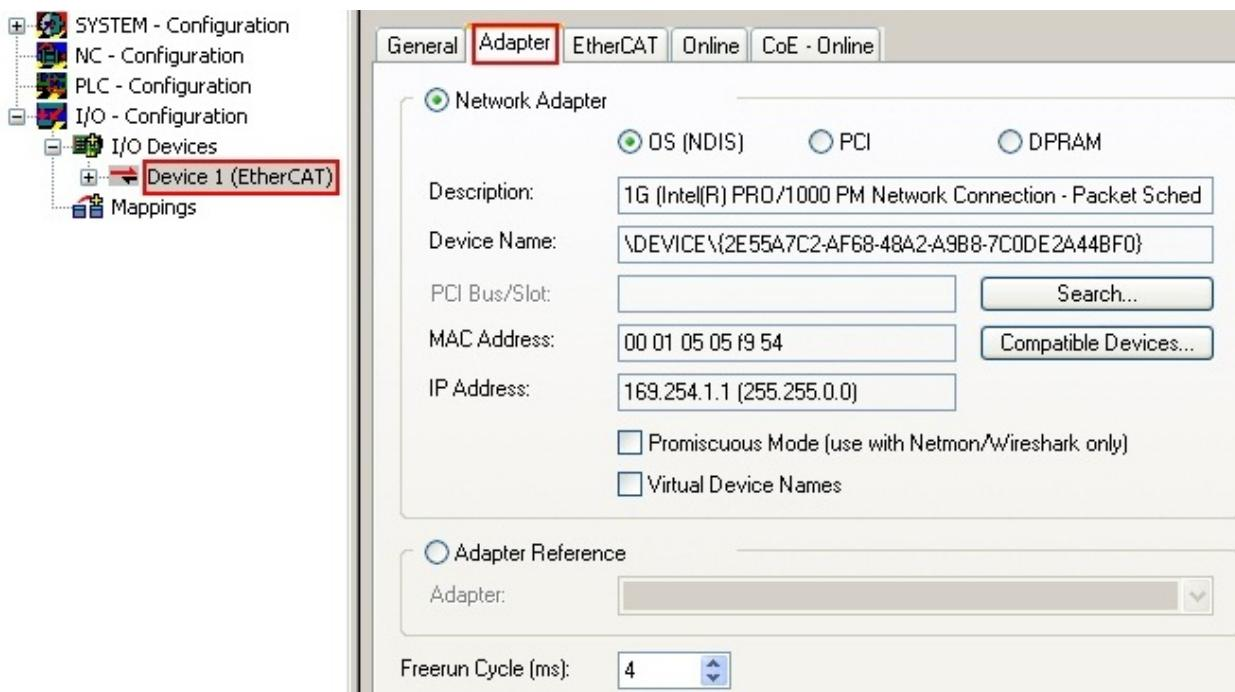
Fig. 77: EtherCAT device properties (TwinCAT 2)
