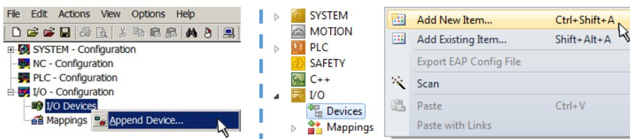
Fig. 74: Append EtherCAT device (left: TwinCAT 2; right: TwinCAT 3)
