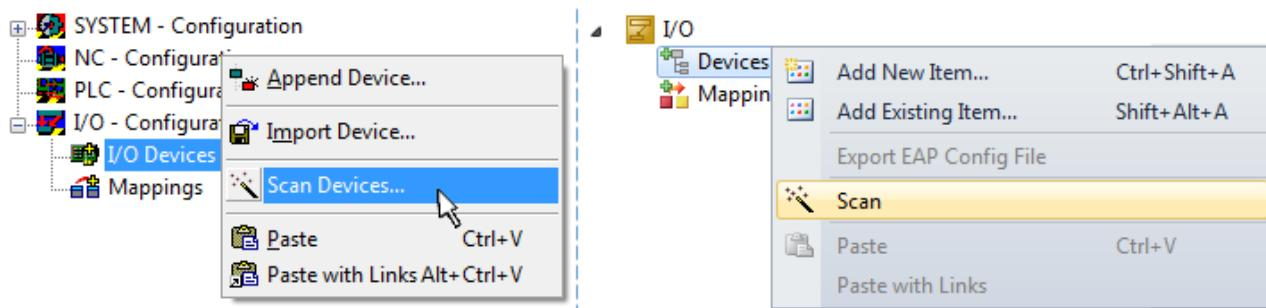
Fig. 85: Scan Devices (left: TwinCAT 2; right: TwinCAT 3)
