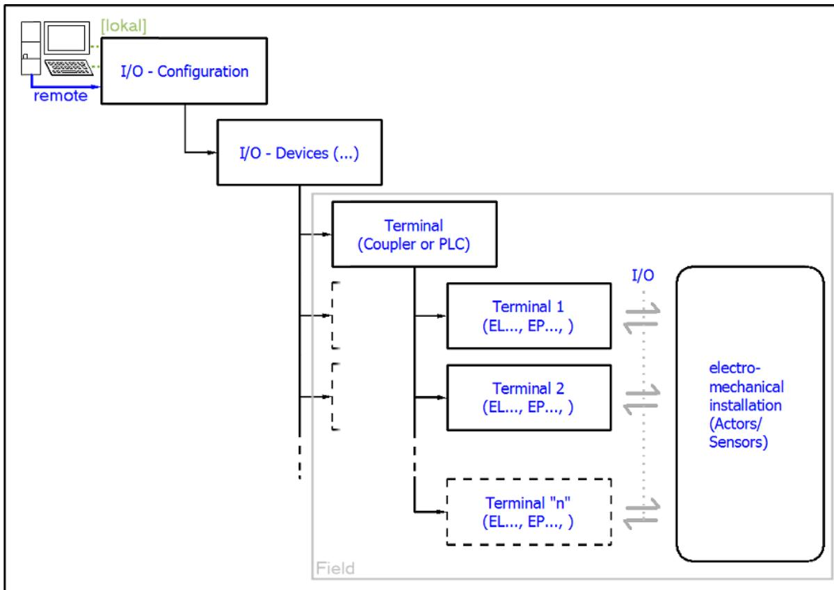
Fig. 17: Relationship between user side (commissioning) and installation
