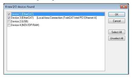
Fig. 35: Automatic detection of I/O devices: selection the devices to be integrated
