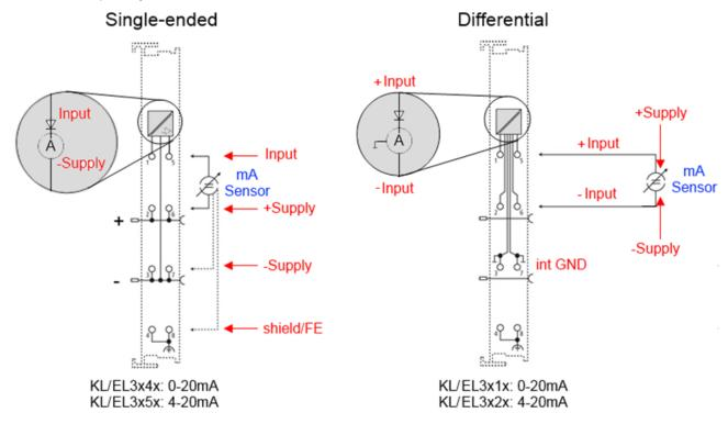
Fig. 174: Connection of externally supplied sensors
