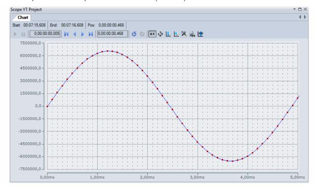
Fig. 147: Example of recording a sine signal with 10 x oversampling at 1 ms measurement cycle time
