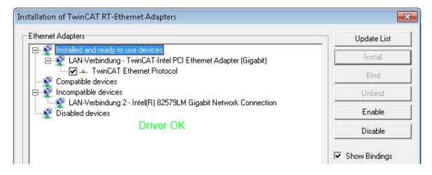
Fig. 76: Exemplary correct driver setting for the Ethernet port
