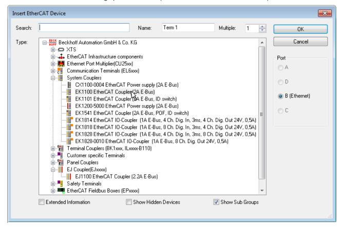
Fig. 92: Selection dialog for new EtherCAT device
