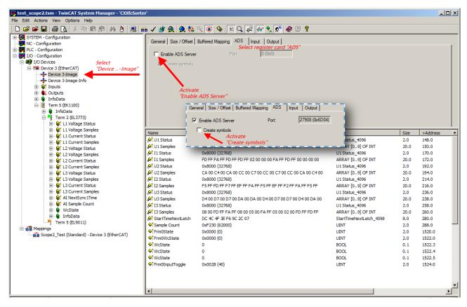
Fig. 163: Activation of the ADS server of the EtherCAT Device (TwinCAT 2)
