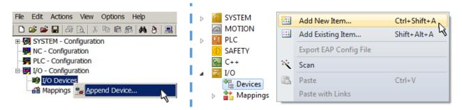
Fig. 87: Append EtherCAT device (left: TwinCAT 2; right: TwinCAT 3)
