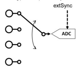
Fig. 183: Schematic representation of multiplex sampling with an ADC converter
