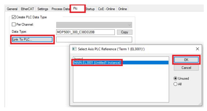
Fig. 68: Linking the structure
