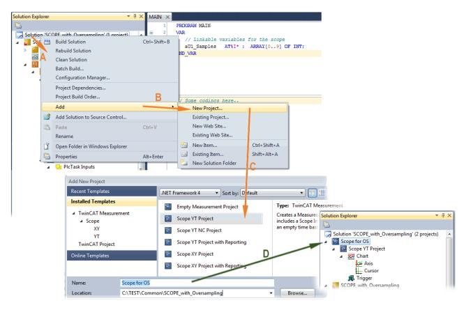
Fig. 138: Adding a Scope project into an already existing project
