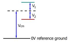
Fig. 176: Common-mode voltage (V<sub>cm</sub>)
