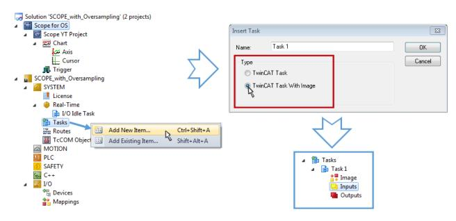
Fig. 140: Insertion of a free task
