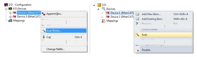
Fig. 105: Manual triggering of a device scan on a specified EtherCAT device (left: TwinCAT 2; right: TwinCAT 3)
