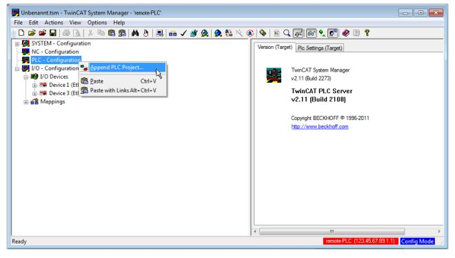
Fig. 40: Appending the TwinCAT PLC Control project
