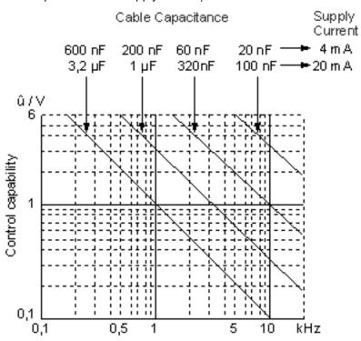
Fig. 6: Control capability of the IEPE impedance transformer depending on cable capacitance and supply current.
