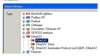
Fig. 88: Selecting the EtherCAT connection (TwinCAT 2.11, TwinCAT 3)
