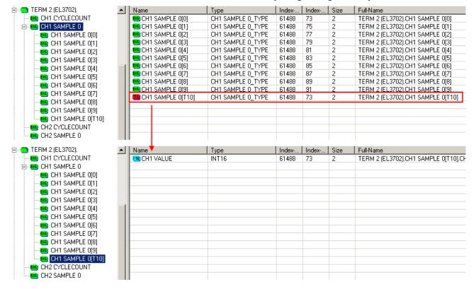
Fig. 165: Automatically calculated array variable (red) in the Scope2
