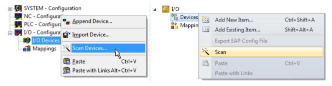
Fig. 98: Scan Devices (left: TwinCAT 2; right: TwinCAT 3)
