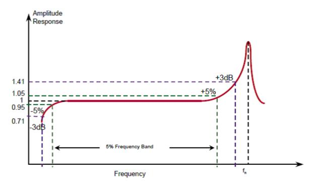
Fig. 8: Frequency response of an acceleration sensor
