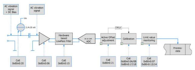
Fig. 166: Data flow of a channel
