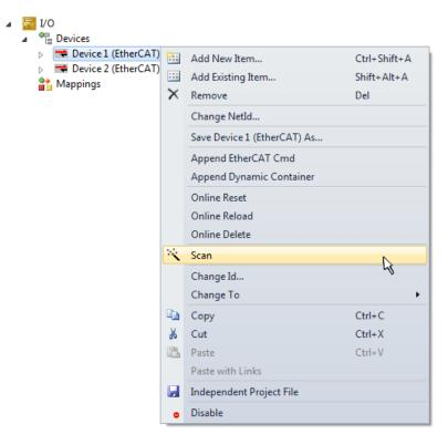
Fig. 56: Reading of individual terminals connected to a device
