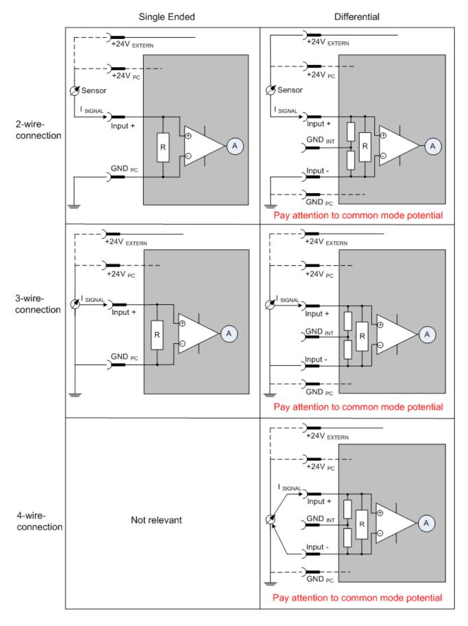
Fig. 175: 2-, 3- and 4-wire connection at single-ended and differential inputs
