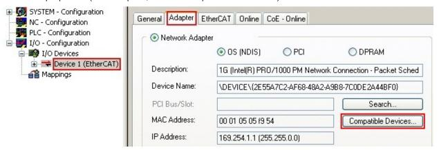
Fig. 74: EtherCAT device properties(TwinCAT 2): click on "Compatible Devices..." of tab "Adapte""
