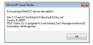
Fig. 84: Information window for faulty ESI file (left: TwinCAT 2; right: TwinCAT 3)
