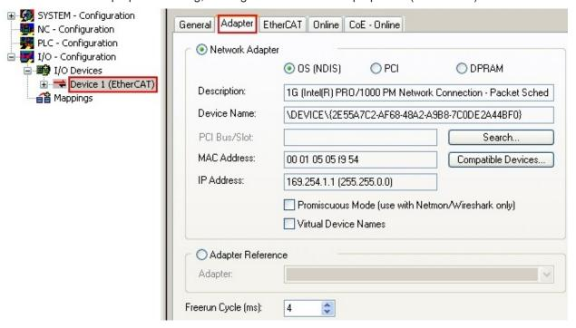
Fig. 90: EtherCAT device properties (TwinCAT 2)
