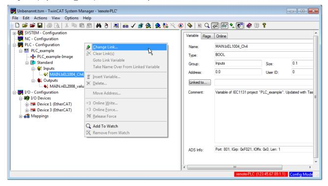
Fig. 42: Creating the links between PLC variables and process objects
