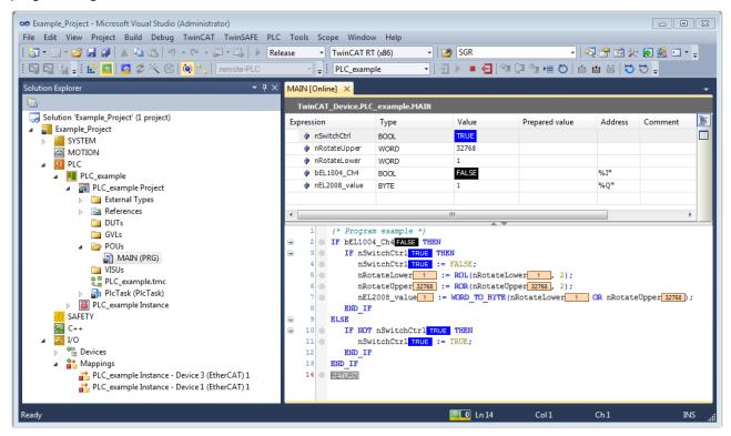
Fig. 70: TwinCAT development environment (VS shell): logged-in, after program startup
