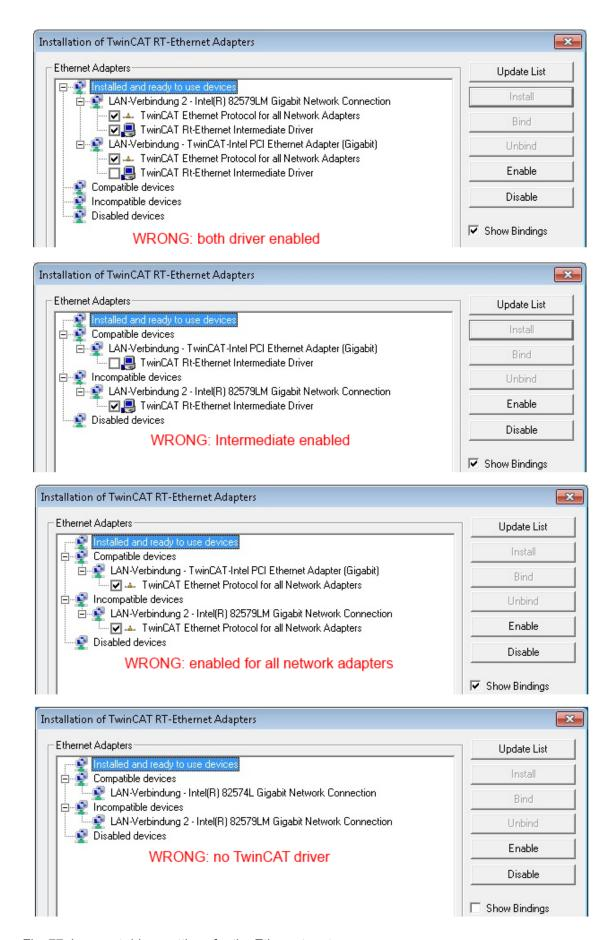
Fig. 77: Incorrect driver settings for the Ethernet port
