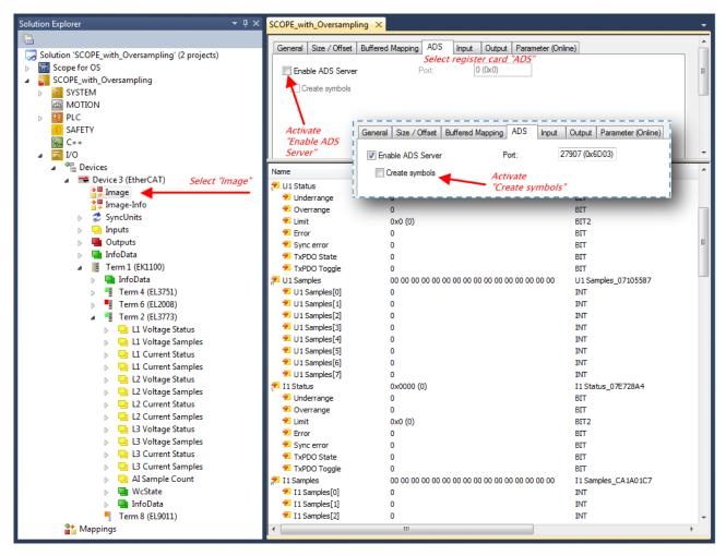
Fig. 148: Activation of the ADS server of the EtherCAT device (TwinCAT 3)
