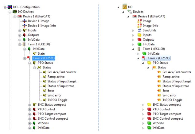
Fig. 96: EtherCAT terminal in the TwinCAT tree (left: TwinCAT 2; right: TwinCAT 3)
