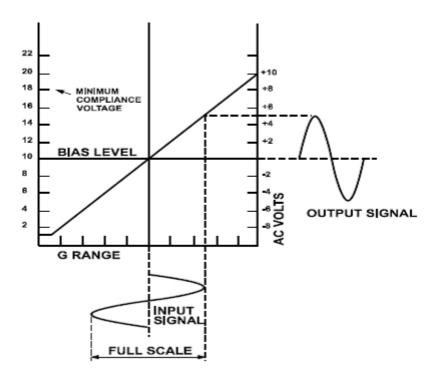
Fig. 7: Output signal of an IEPE sensor (sample)
