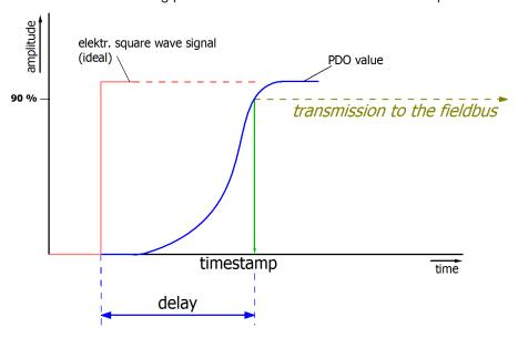
Fig. 179: Diagram signal delay (step response)
