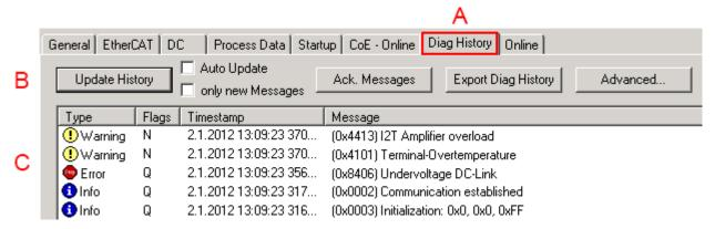
Fig. 187: Implementation of the DiagMessage system in the TwinCAT System Manager
