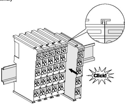
Fig. 18: Attaching on mounting rail
