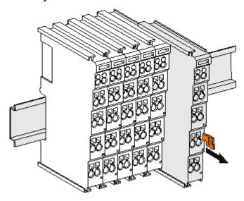
Fig. 19: Disassembling of terminal
