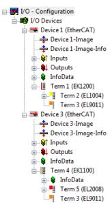
Fig. 36: Mapping of the configuration in the TwinCAT 2 System Manager
