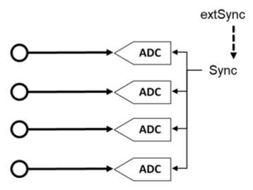
Fig. 182: Schematic representation simultaneous sampling with 4 ADC converters
