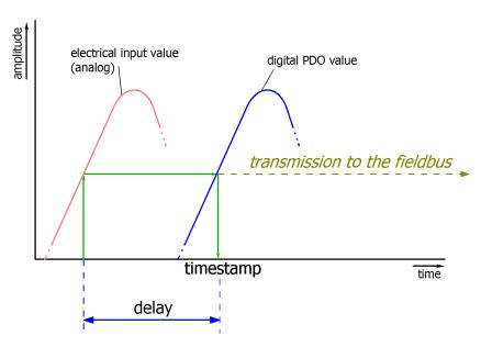
Fig. 180: Diagram signal delay (linear)
