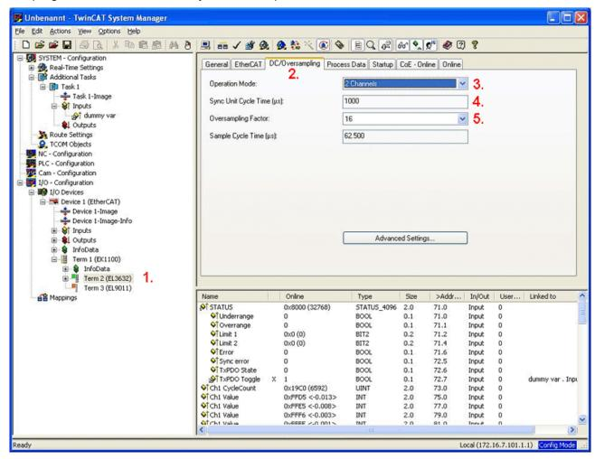
Fig. 169: Setting the sampling rate in TwinCAT
