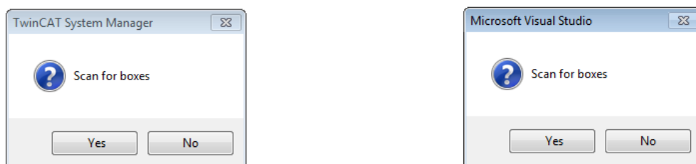
Fig. 61: Scan query after automatic creation of an EtherCAT device (left: TwinCAT 2; right: TwinCAT 3)
