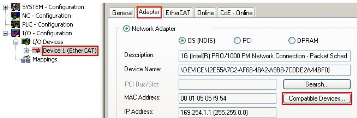
Fig. 72: EtherCAT device properties(TwinCAT 2): click on “Compatible Devices...” of tab “Adapte””
