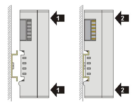
and press (1) the terminal module against the mounting rail until it latches in place on the mounting rail (2).
