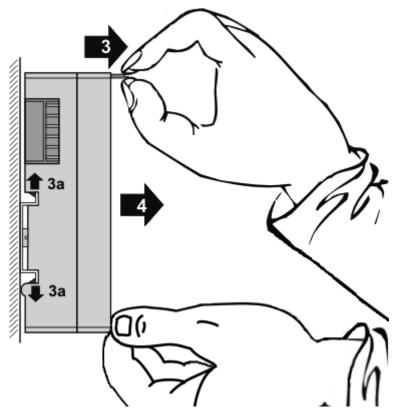
• Pull (4) the terminal module away from the mounting surface. Avoid canting of the module; you should stabilize the module with the other hand, if required.
