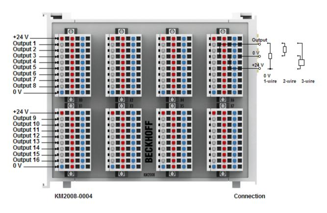
Fig. 10: Digital Terminal Modules with 64 output channels
