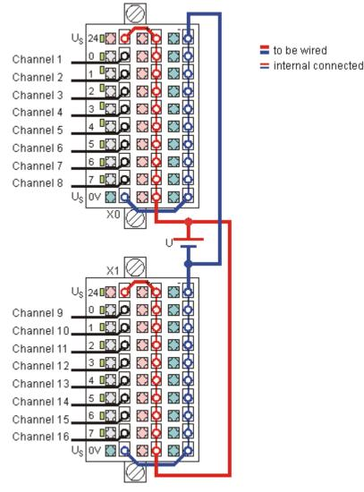
Fig. 17: Supply voltage connection
