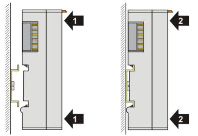
and press (1) the terminal module against the mounting rail until it latches in place on the mounting rail (2).
