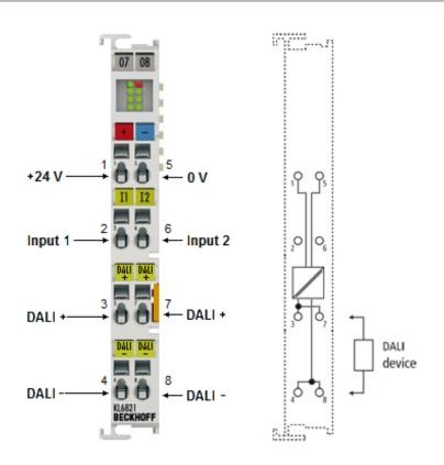
Fig. 11: KL6821 - Contact assignment
