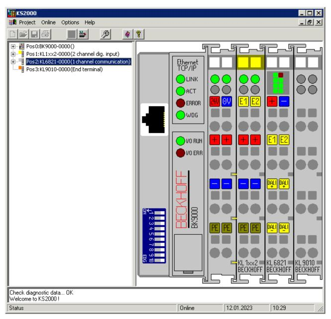
Fig. 14: Display of the fieldbus station in KS2000
