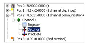
Fig. 15: KS2000 tree branches for channel 1 of the KL6821
