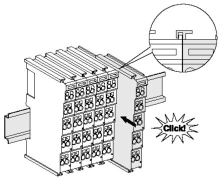
Fig. 4: Attaching on mounting rail
