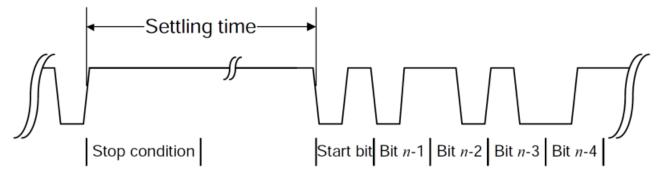
The length of the *settling time* depends on the DALI priority with which a data frame is sent. The higher the DALI priority, the smaller the *settling time*.
