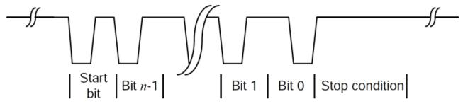
Transmission is via Manchester coding with a data transfer rate of 1200 bits per second. Thus, each bit has a length of 0.833 ms (1 / 1200 = 0.000833).
