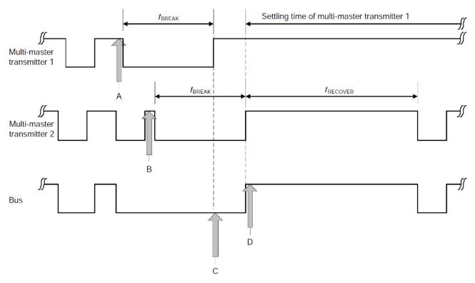
The break sequence has a length of 1.2 ms to 1.4 ms, while the recover sequence can be between 4.0 ms and 4.6 ms.
