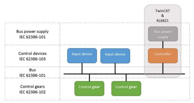
Up to 64 DALI control gears and up to 64 DALI control devices can be connected to the KL6821 per DALI line. The KL6821 represents the DALI controller. One such device exists for each DALI line. Up to 64 control gears, which have to be DALI/DSI devices, can be connected to the KL6811. Any number of DALI lines (KL6821 and KL6811) can be operated with a single TwinCAT controller.
