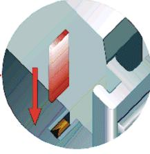
Fig. 6: Power contact on left side
