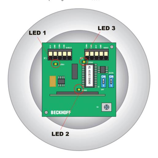
Fig. 5: KL6583 - Diagnostic LEDs
