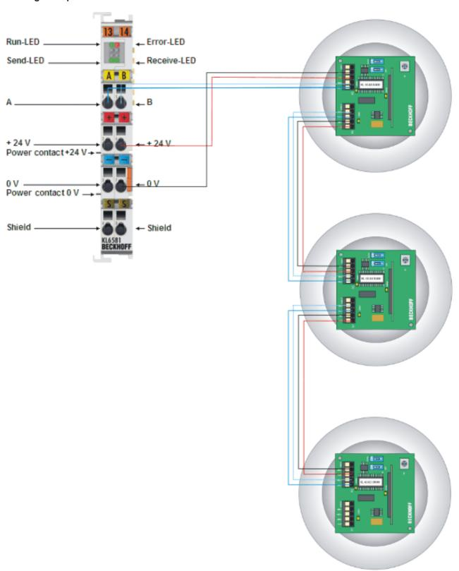
Fig. 19: KL6581, KL6583 - cabling example
