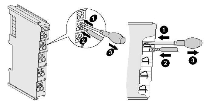
Fig. 13: Connecting a cable on a terminal point
