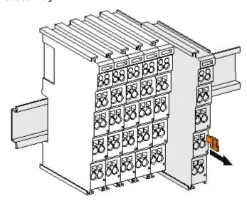
Fig. 8: Disassembling of terminal
