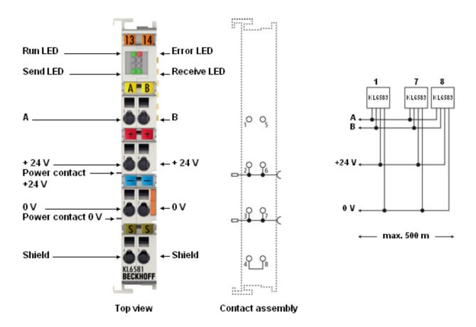
Fig. 14: KL6581 - Contact assignment
