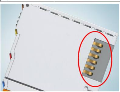
Fig. 6: Spring contacts of the Beckhoff I/O components
