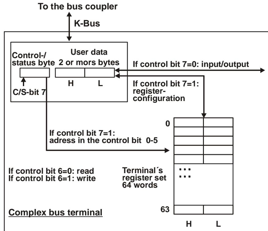
The control or status byte occupies the lowest address of a logical channel. The corresponding register values are located in the following 2 data bytes (the BK2000 is an exception to the rule: here, an unused data byte is inserted after the control or status byte, thus setting the register value to a word limit).
