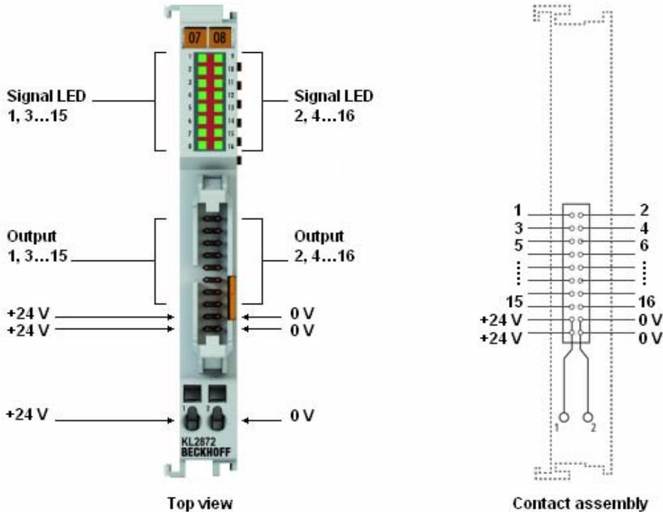
**Sixteen channel digital output terminal with flat ribbon cable connection, 24 V<sub>DC</sub>**
