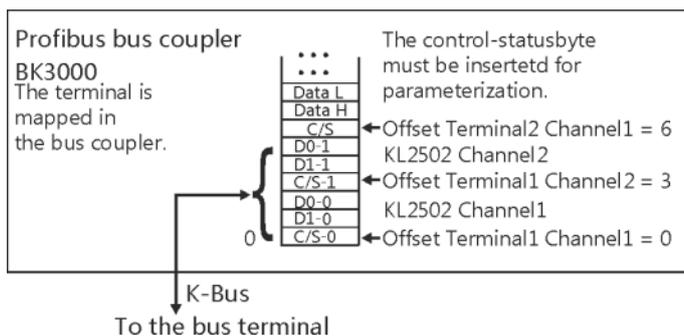
Fig. 15: Mapping in the Profibus coupler – example for KL2502
