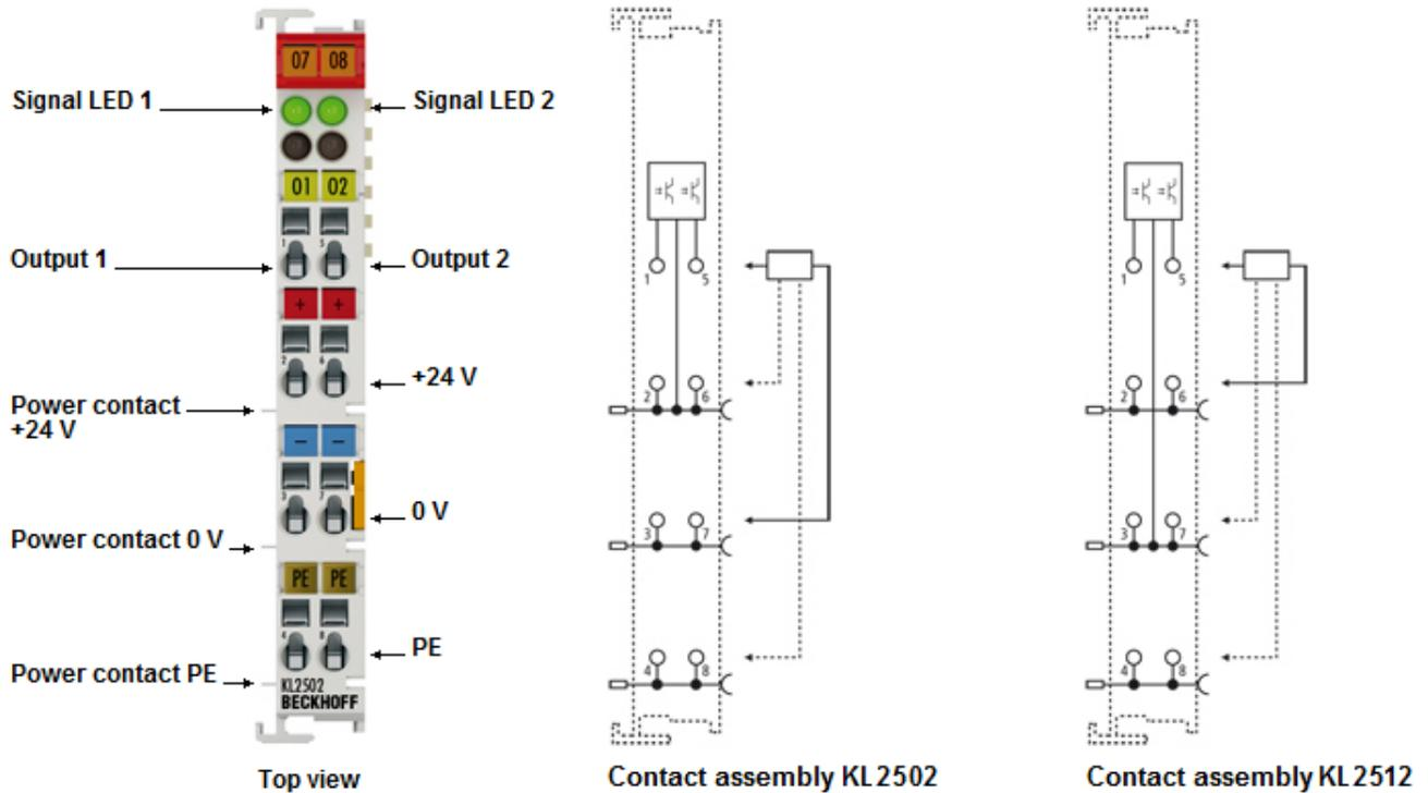
Fig. 12: KL2502, KL2512 - Contact assignment and LEDs
