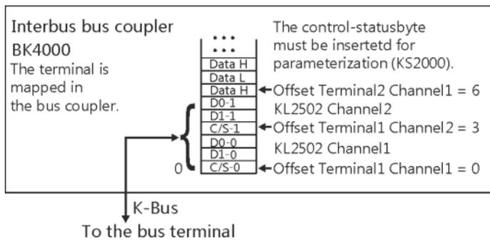
Fig. 16: Mapping in the Interbus coupler – example for KL2502
