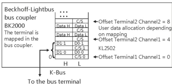
Fig. 14: Mapping in the Lightbus coupler – example for KL2502
