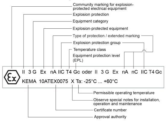
Fig. 1: Marking of equipment
