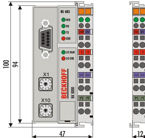
The overall width of the construction is the width of the bus coupler, including the bus end terminal, plus the width of the installed bus terminals. The bus terminals are 12 mm or 24 mm wide, depending on their function. Depending on the gauge of cables used the overall height of 68 mm may be overstepped by about 5 mm to 10 mm by the cables at the front.
