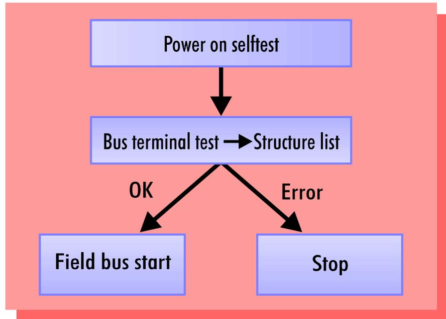
The bus coupler reports the error to the master by means of the Profibus diagnostics. Clearing the error returns the bus coupler to its normal operating mode.
