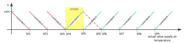
In this diagram controller 4 would be placed incorrectly, if controller 5 changed to heating mode. Or: Controller 4 is correct, but controller 5 would have to be a pure cooling controller. In both cases there would be two switches from heating to cooling.
