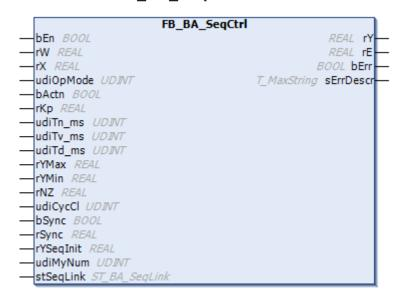
PID controller as part of a sequence.
