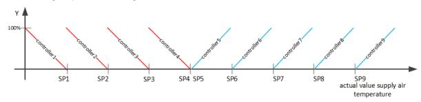
A series of heating sequences should not include a cooling sequence. Similarly, a series of cooling sequences should not include a heating sequence. Sequences with reversal of direction of action for a mixed air system or heat recovery should be positioned between the heating and cooling sequences.
