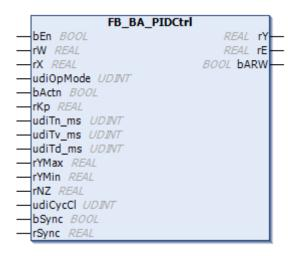
Universal PID controller, alternatively in parallel structure or with upstream proportional component.
