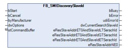
The first drive is sought that corresponds to the specified manufacturer code and has the address 0. This function block is used in the addressing of SMI devices and is used in the <u>FB\_SMIAddressing() [▶ 35]</u> function block.
