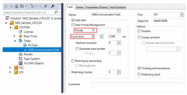
Add the program for the communication to this task. More precise information on the task configuration can be found in the function block description.
