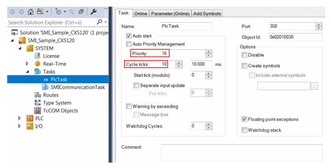
Create a further task for the background communication. Assign a higher priority (smaller number) and a lower interval time to this task than the PlcTask.
