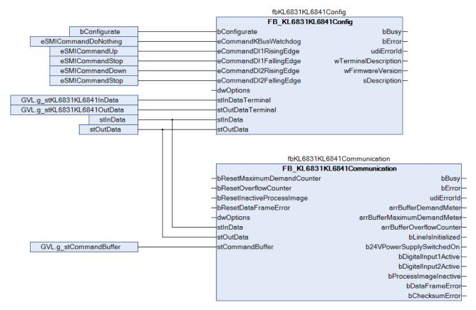
The function block FB\_KL6831KL6841Config() is linked to the process image of the KL6831/KL6841. Once the configuration is complete, the function block <u>FB\_KL6831KL6841Communication()</u> [▶ 12] received the process values of the KL6831/KL6841. No SMI commands can be sent while the configuration is in progress.
