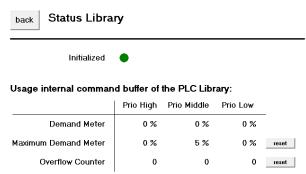
Communication between the individual PLC blocks and the Bus Terminal takes place within the PLC library via three central buffers (for each SMI terminal). The extent of utilisation of the buffers and possible overflows can be determined from the illustrated table.
