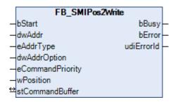
Writes the fixed position *Pos2* which is configurable on the motor side. *Pos2* can be changed using the <u>FB SMIPos2Read() [ > 27]</u> block.
