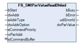
Reads a DWord parameter (4 bytes) stored on the motor side. The meaning of the individual parameters is manufacturer-specific.
