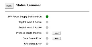
The status information from the process image of the terminal is displayed in this dialogue. In addition, messages requiring acknowledgement can be reset in this dialogue.
