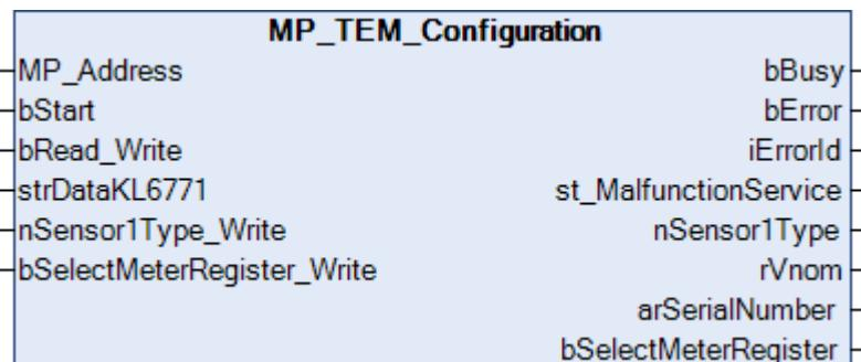
This function block is used to configure the Thermal Energy Meter type 22PE-.. and 22PEM-... . For more information please visit [www.belimo.com](http://www.belimo.com).
