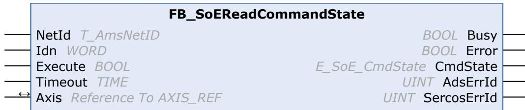
With the FB\_SoEReadCommandState function block the command execution can be checked.
