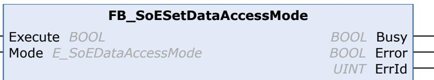
The SoE parameter access mode is set with the function block FB\_SoESetDataAccessMode. Attributes & Value are accessed in parallel by default. If this access mode is not supported by the device manufacturer, sequential access can be enforced. Generally, however, parallel access is faster.
