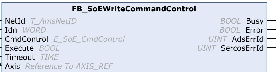
With the FB\_SoEWriteCommandControl function block a command can be prepared, started or canceled.
