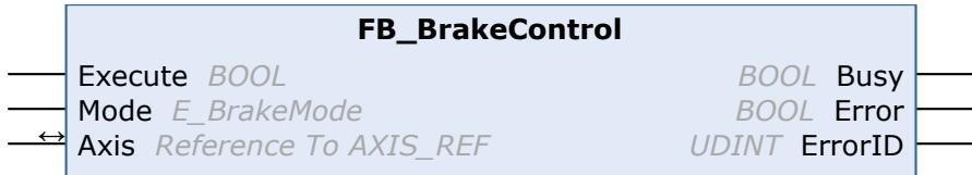
The FB\_BrakeControl function block can be used to manually open or close the brake of a motor that is operated on Beckhoff servo hardware.
