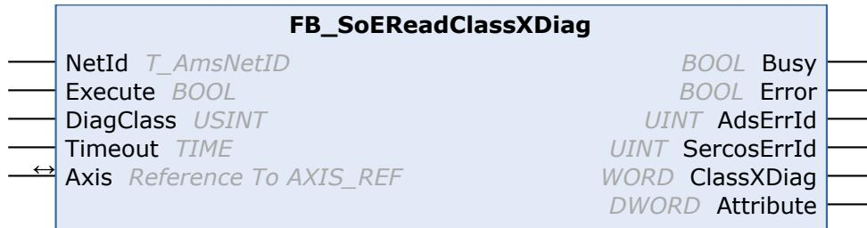
With the function block FB\_SoEReadClassXDiag, the current Class 1 diagnosis (S-0-0011) ... Class 3 diagnosis (S-0-0013) can be read out as WORD. There is the conversion function F\_ConvWordToSTAX5000C1D for the evaluation of the Class 1 diagnosis as a structure ST\_AX5000\_C1D, (see TwinCAT 3 PLC Lib Tc2\_Drive documentation).
