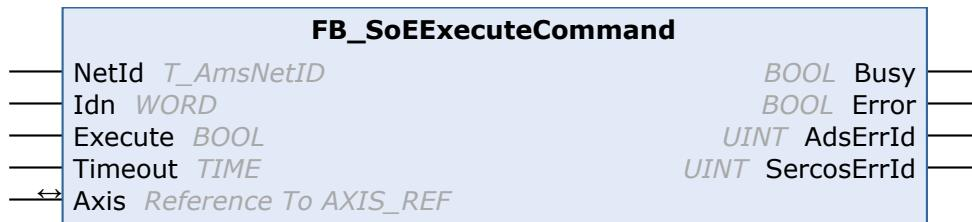
With the FB\_SoEExecuteCommand function block a command can be executed.
