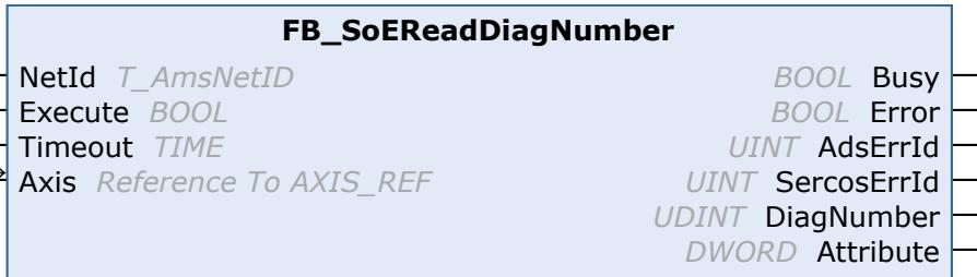
With the FB\_SoEReadDiagNumber function block the current diagnostic number can be read out as UDINT (S-0-0390).
