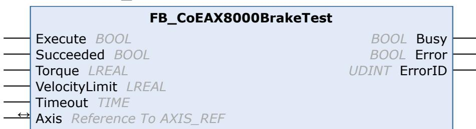
The function block FB\_CoEAX8000BrakeTest can be used to implement a functional brake test.
