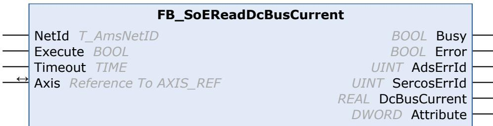
With the FB\_SoEAX5000ReadDcBusCurrent function block the DC-Bus current (S-0-0381) can be read.
