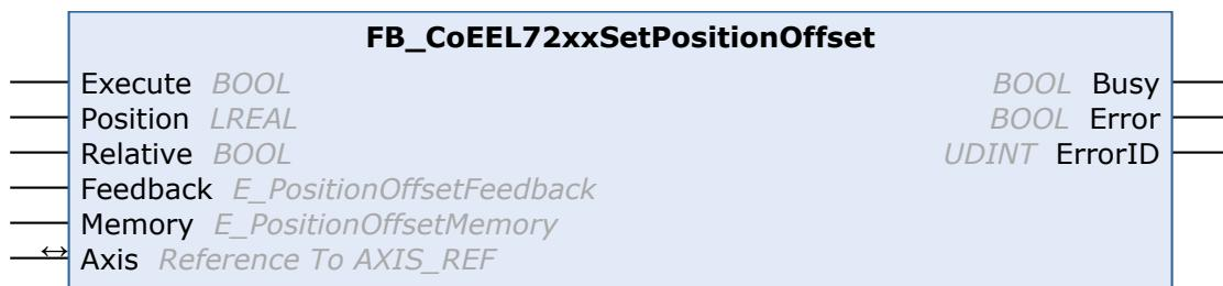
With the function block FB\_CoEEL72xxSetPositionOffset, a position offset can be stored in the memory of the EL72xx. Saving in the digital name plate of the connected motor encoder is not currently provided for.
