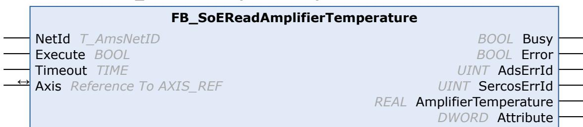
With the FB\_SoEReadAmplifierTemperature function block the temperature of the drive (S-0-0384) can be read.
