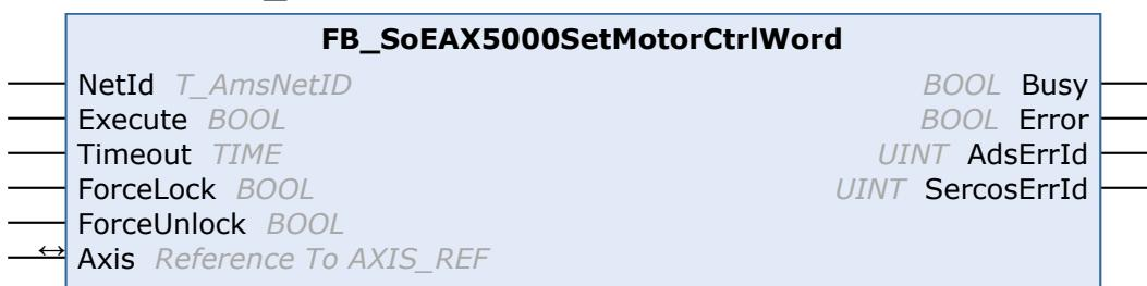
With the FB\_SoEAX5000SetMotorCtrlWord function block the ForceLock bit (Bit 0) or the ForceUnlock bit can be set in the Motor Control Word (P-0-0096) to activate or release the brake. Normally the brake is automatically controlled via the Enable of the drive.
