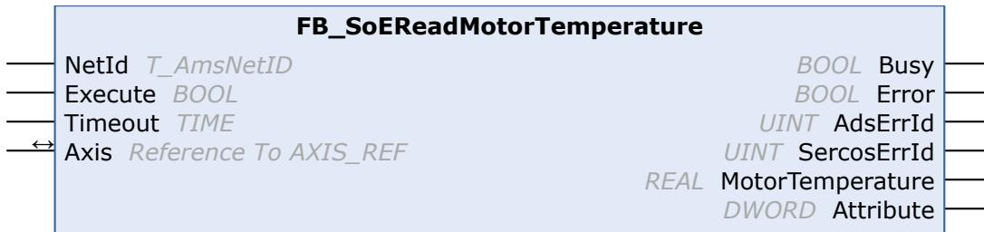
With the function block FB\_SoEReadMotorTemperature the temperature of the motor (S-0-0383) can be read. If the motor does not contain a temperature sensor, this is 0.0, i.e. 0.0 °C.
