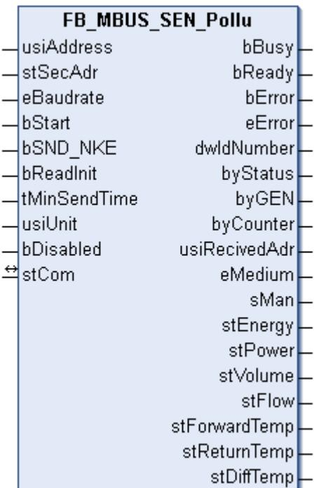
This block is used for reading heat/cold meters from Sensus:
