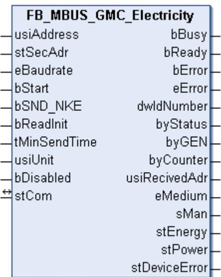
This block is used to read electricity meters from Gossen Metrawatt:
