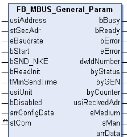
This block is used for reading any M-Bus devices. The variable [arrData](#) [▶ 204] supplies [cMBUS\\_MaxDataParam](#) [▶ 208] values.
