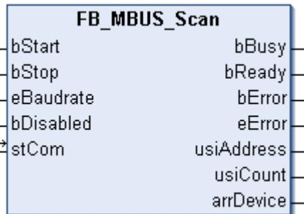
This block can be used to scan the M-Bus bus. All primary addresses (0..250) are queried successively. The array *arrDevice* is used to show certain device information.
