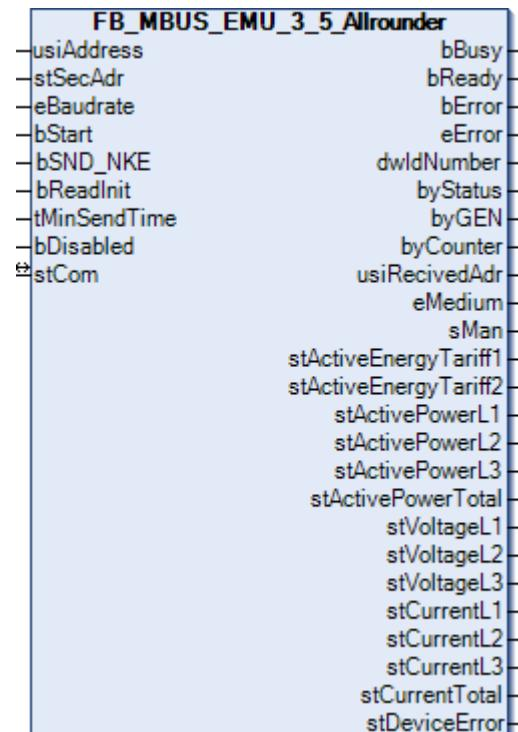
This block is used to read electricity meters from EMU.
