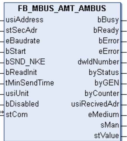
This block is used to read pulse collectors from Aquametro:
