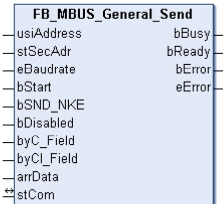
This block serves to send data to any M-Bus devices. (for example, the primary address of the meter can be changed with this block)
