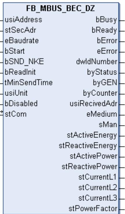
This block is used to read electricity meters from Berg:
