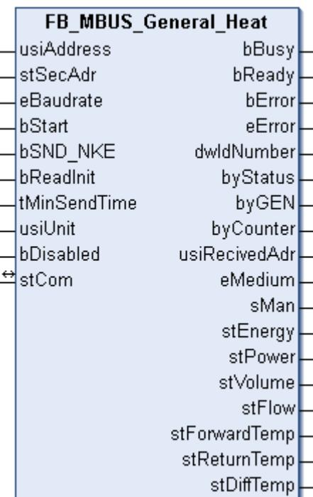
This block is used to read heat meters.
