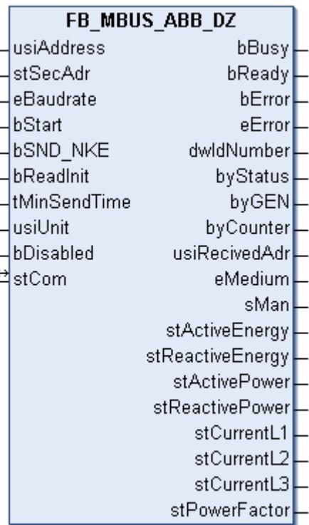
This block is used to read electricity meters from ABB:
