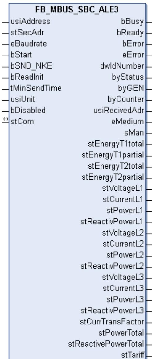
This block is used to read electricity meters from Saia-Burgess:
