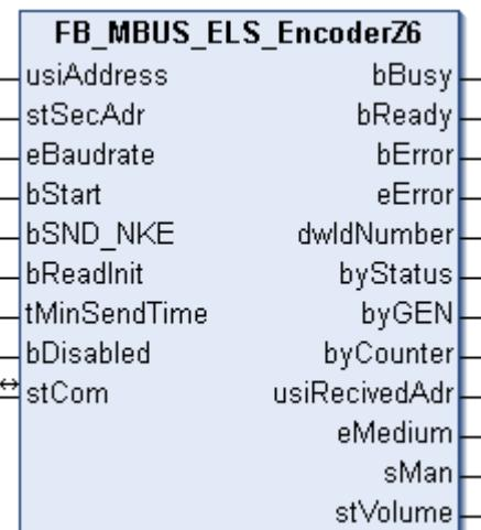
This block is used to read meters from Elster:
