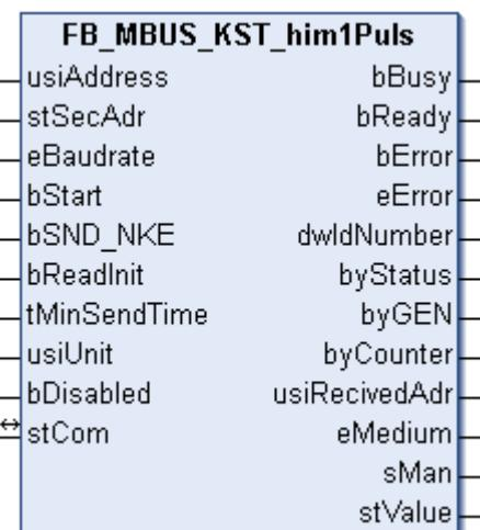
This block is used for reading M-Bus modules from KUNDO System Technik:
