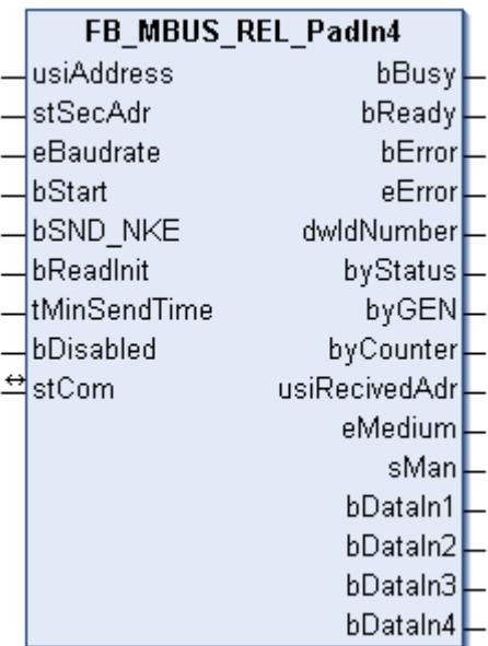
This block is used for reading digital inputs from Relay:
