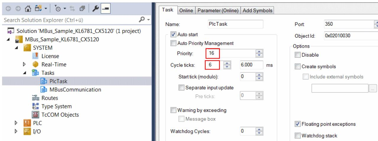
Create a further task for the background communication. Assign a higher priority (smaller number) and a lower interval time to this task than the PLCTask.
