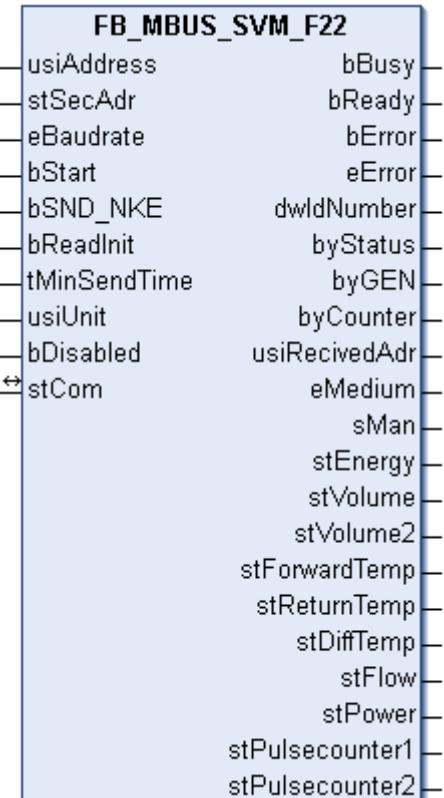
This block is used to read heat meters from Metrima:
