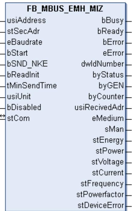
This block is used to read electricity meters from EMH:
