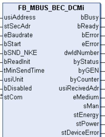
This block is used to read electricity meters from Berg:
