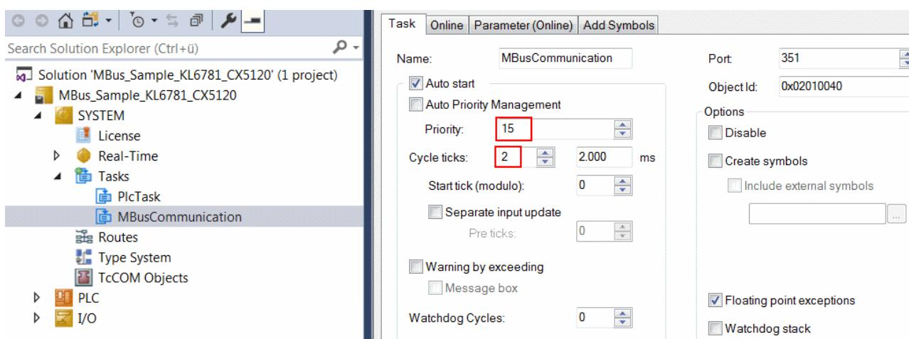
Add the program for the communication to this task. Further information on task configuration can be found in the description of the function block [FB\\_MBUSKL6781 \[▶ 19\]](#).
