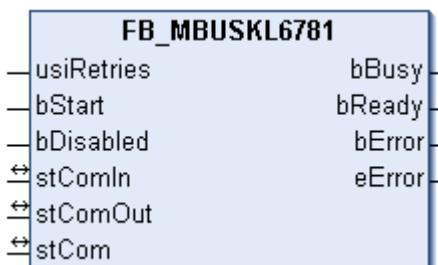
This function block is used to read M-Bus devices via the Bus Terminal KL6781.
