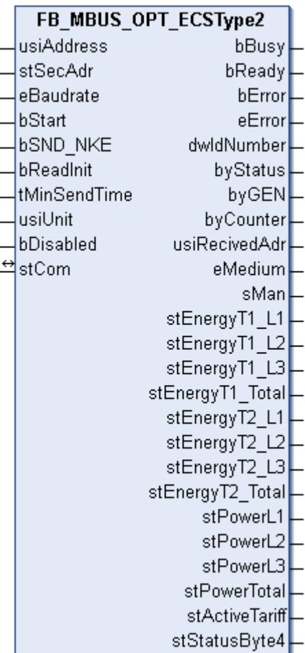
This block is used to read electricity meters from OPTEC:
