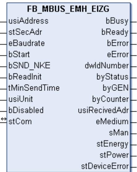
This block is used to read electricity meters from EMH:
