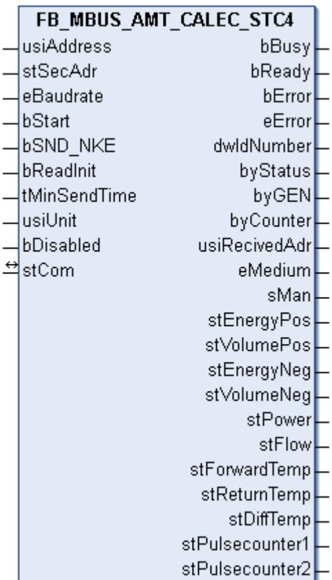
This block is used to read heat meters from Aquametro:
