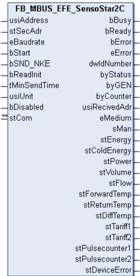
This block is used to read heat meters from Engelmann:
