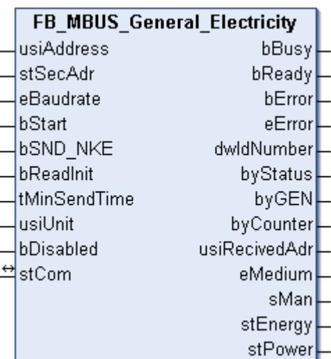
This block is used to read electricity meters.
