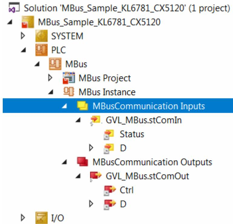
Now link the global variables of PLC program with the inputs and outputs of the Bus Terminals. Create the Solution and enable the configuration.
