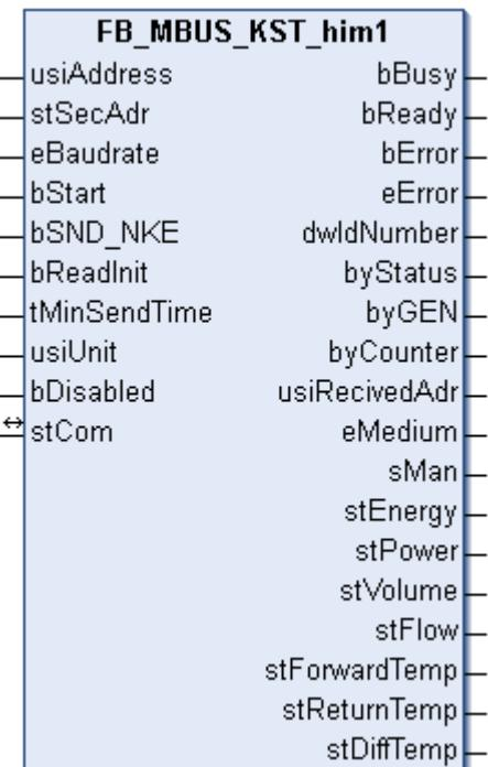
This block is used for reading M-Bus modules from KUNDO System Technik:
