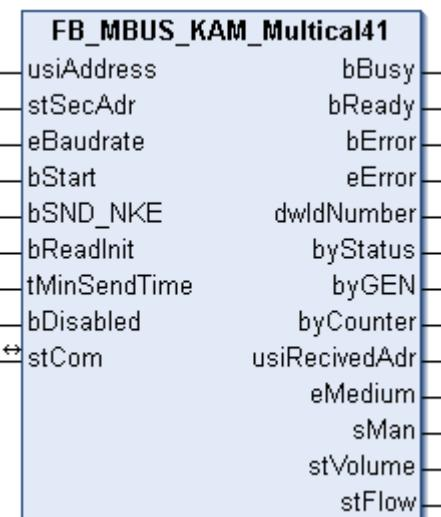
This block is used to read water meters from Kamstrup:
