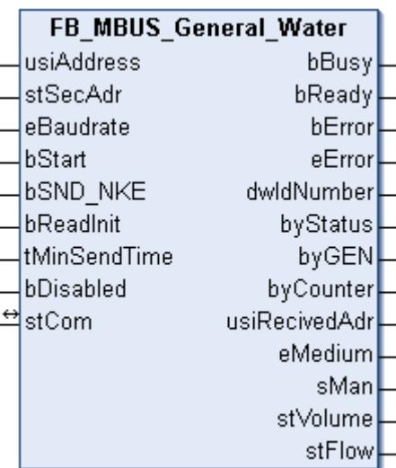
This block is used to read water meters.
