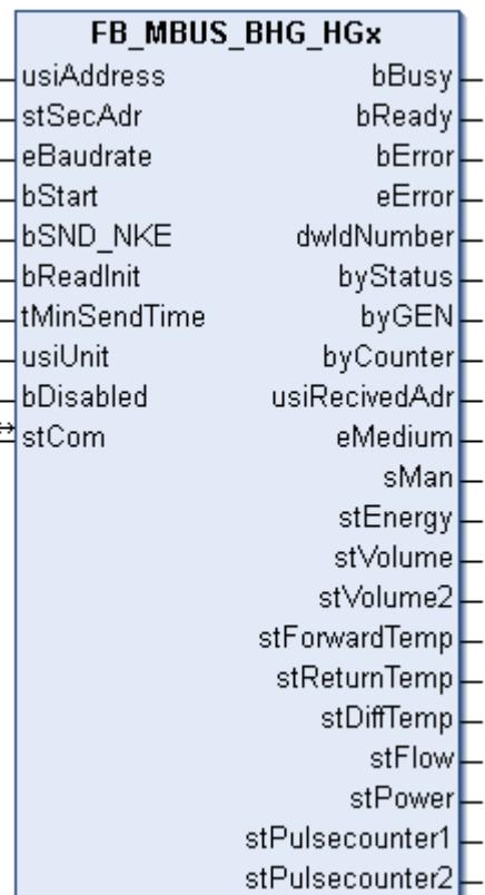
This block is used to read heat meters from Brunata:
