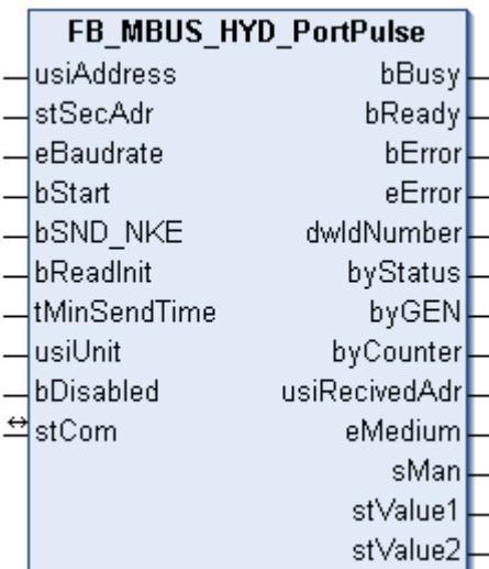
This block is used for reading energy meters with pulse output from Hydrometer:
