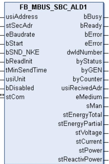
This block is used to read electricity meters from Saia-Burgess:
