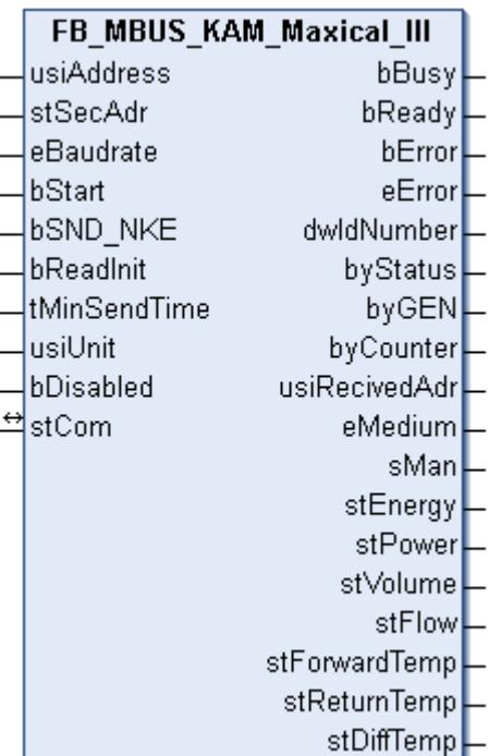
This block is used for reading heat/cold meters from Kamstrup:
