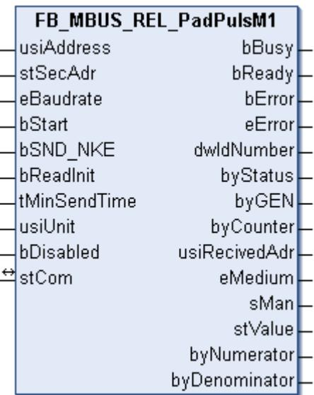
This block is used for reading energy meters with pulse output from Relay:
