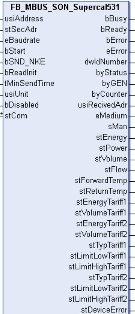
This block is used for reading heat/cold meters from Sontex:
