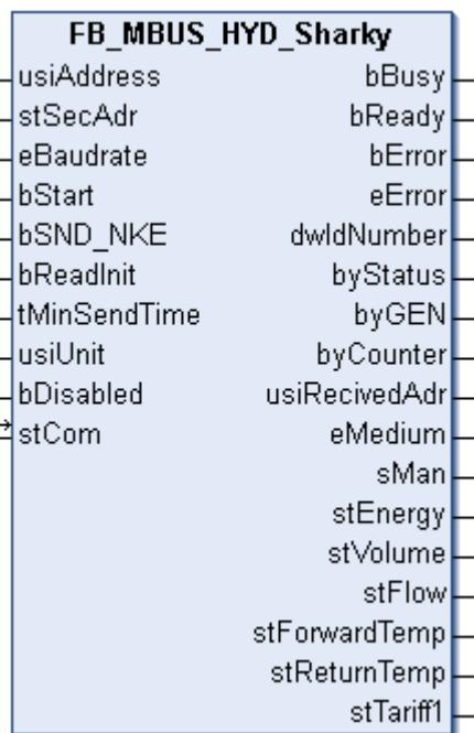
This block is used to read energy meters from:
