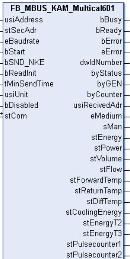
This block is used for reading heat/cold meters from Kamstrup:
