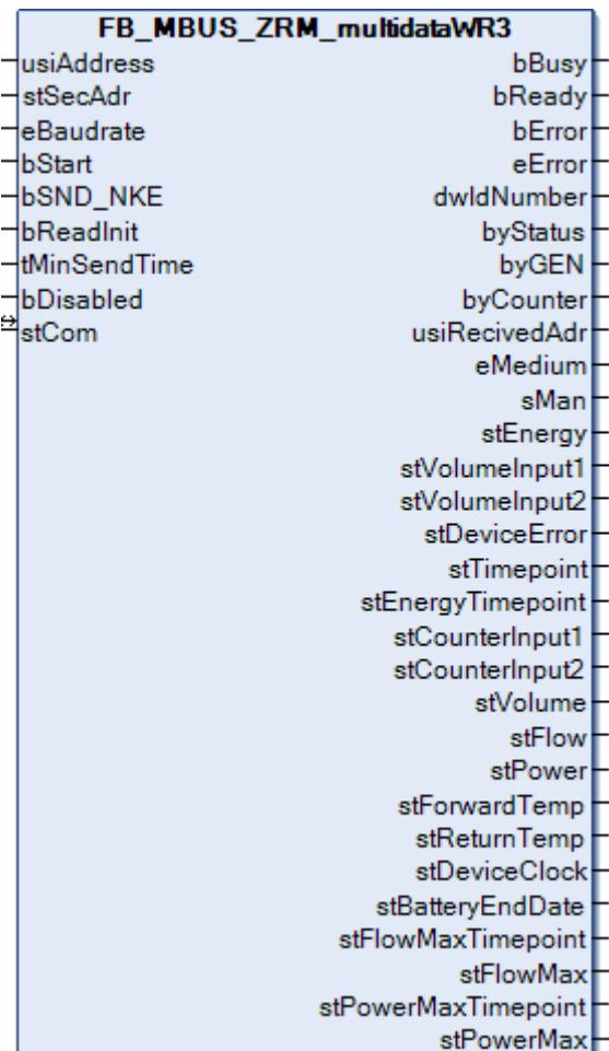
This block is used to read arithmetic units from Zenner.
