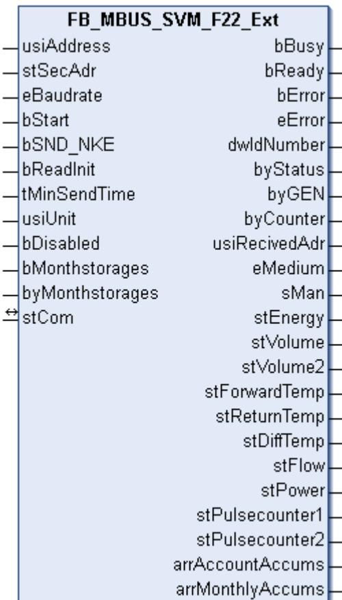
This block is used to read heat meters from Metrima:
