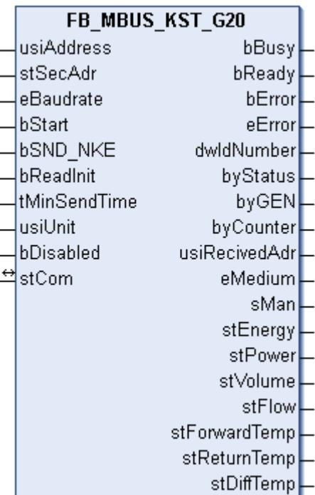
This block is used for reading heat/cold meters from KUNDO System Technik:
