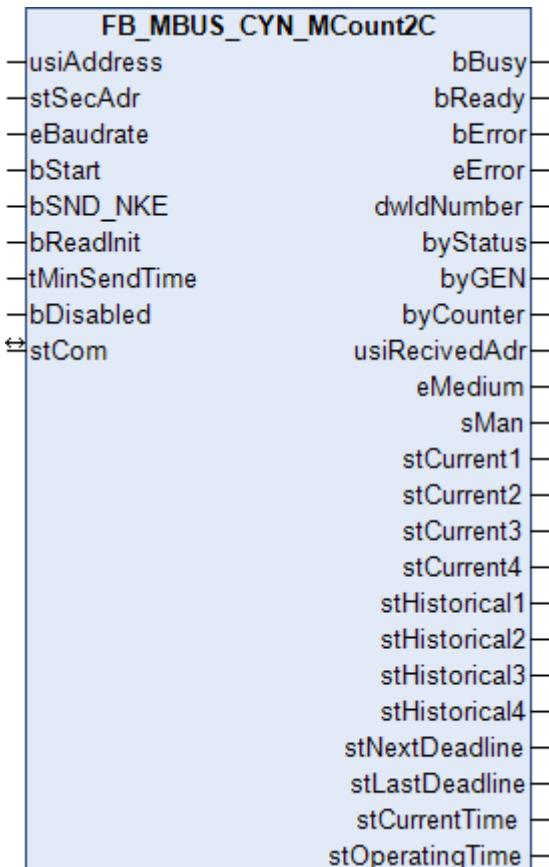
This function block is used to read pulse counters from Cynox.
