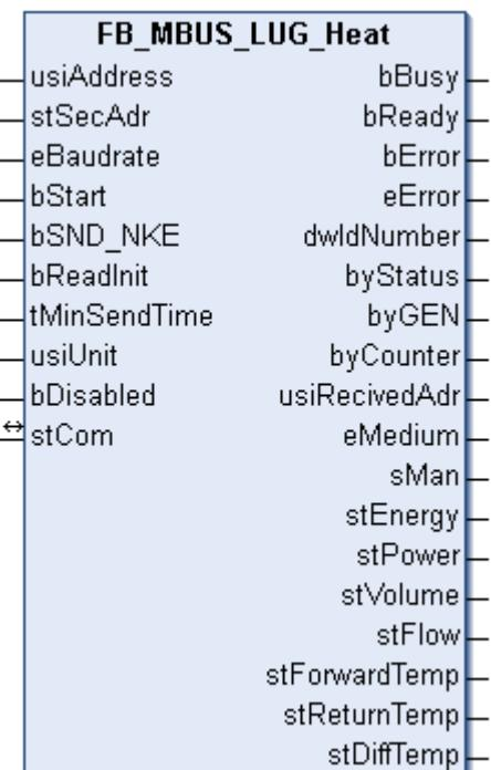
This block is used for reading heat/cold meters from Landis & Gyr:
