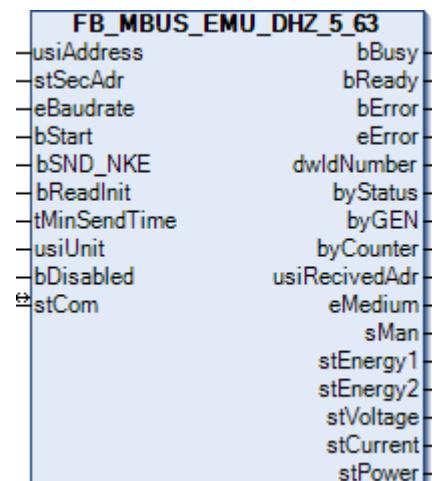
This block is used to read electricity meters from EMU.
