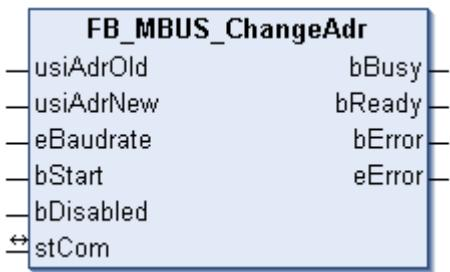
This block can be used to change the primary address.
