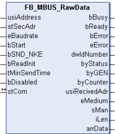
This block is used for reading any M-Bus devices. The variable *arrData* supplies the raw data of the M-Bus device. Only the first telegram is evaluated.
