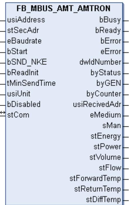
This block is used to read heat meters from Aquametro:
