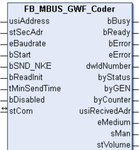
This block is used to read meters from GWF:
