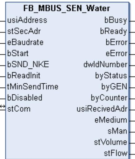
This block is used to read water meters from Sensus.
