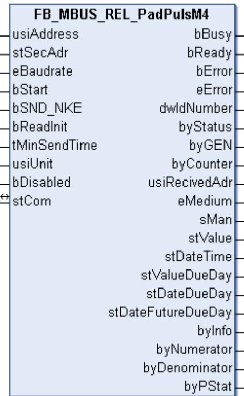
This block is used for reading energy meters with pulse output from Relay:
