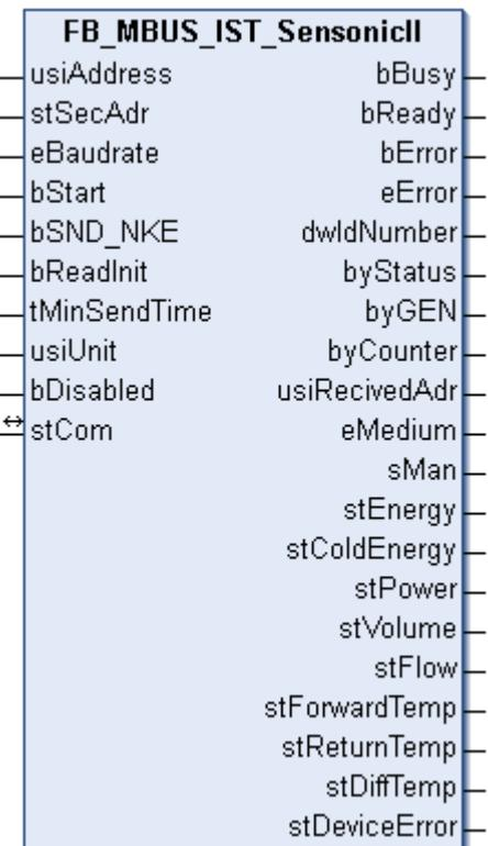
This block is used to read heat meters from Ista:
