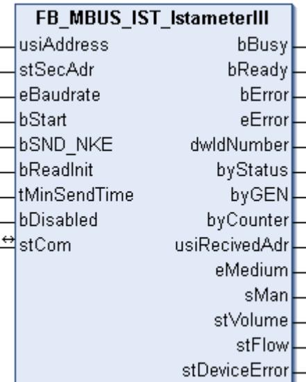
This block is used to read water meters from Ista:
