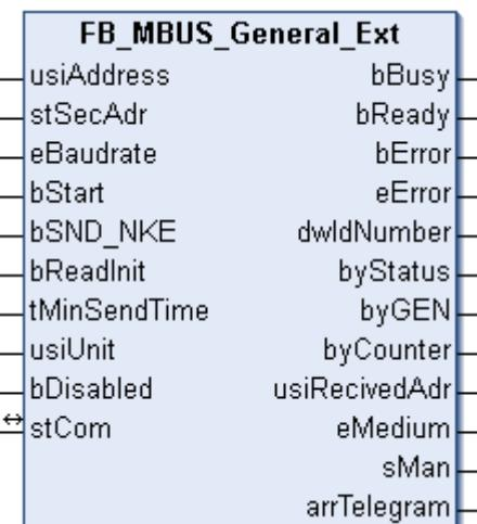
Some M-Bus devices send values distributed over several telegrams. This block can be used to read all telegrams from any M-Bus devices.
