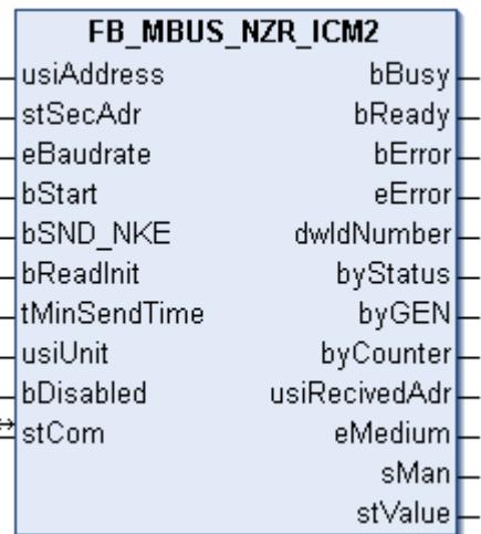
This block is used to read energy meters with pulse output from NZR:
