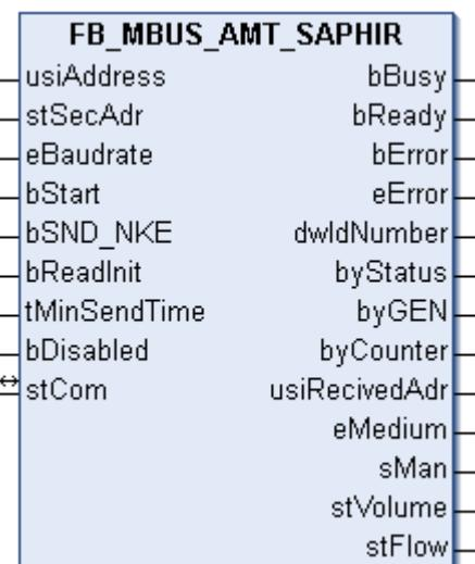
This block is used to read water meters from Aquametro.
