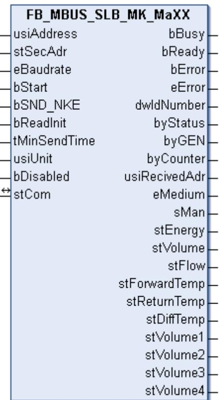
This block is used to read heat meters from Schlumberger:
