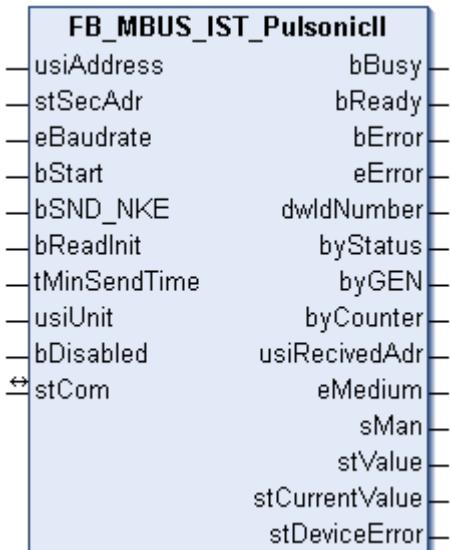
This block is used to read energy meters with pulse output from Ista:
