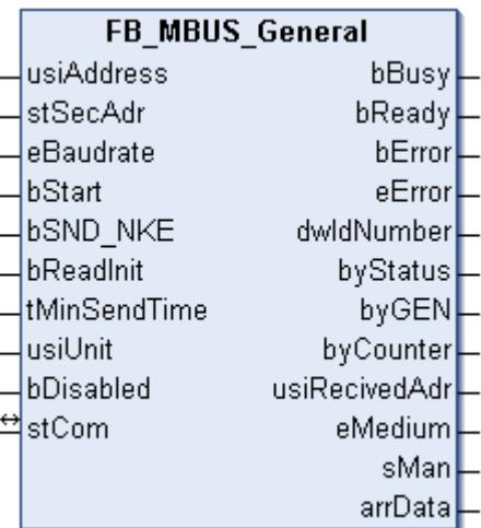
This block is used for reading any M-Bus devices. The variable [arrData \[▶ 204\]](#) supplies a maximum of [cMBUS\\_MaxData \[▶ 208\]](#) values for the first telegram. String values and manufacturer-specific information are not shown correctly.
