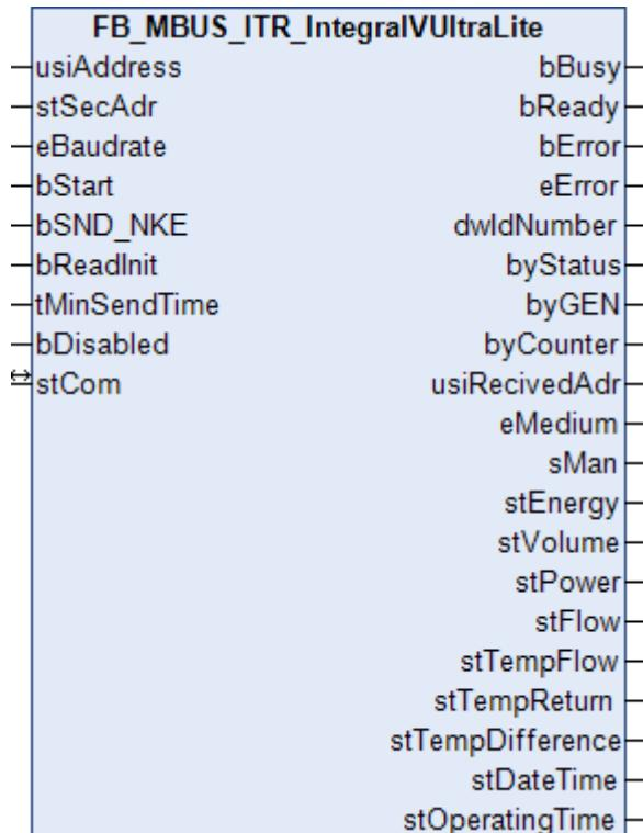
This function block is used to read energy meters from Itron.
