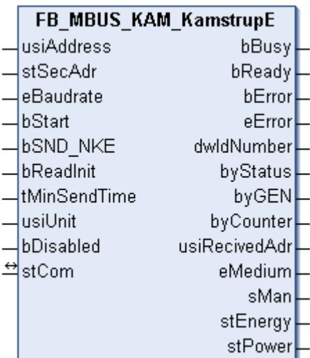
This block is used to read electricity meters from Kamstrup:
