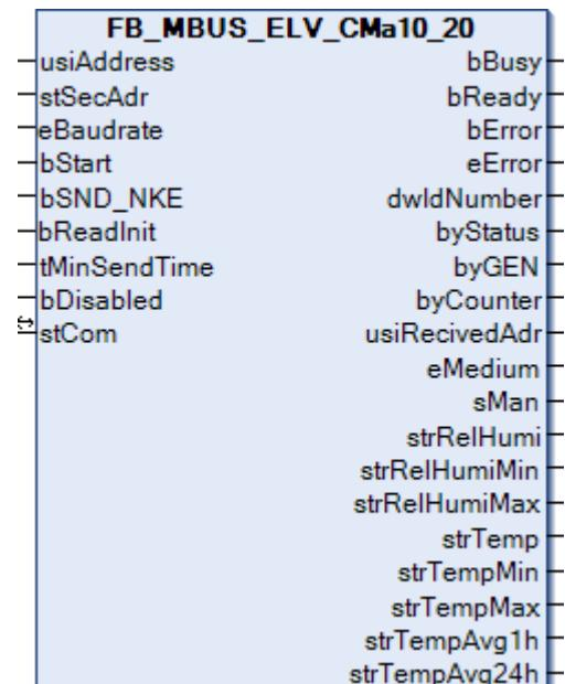
This block is used to read temperature and humidity sensors from elvaco.
