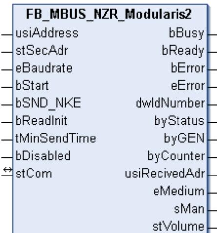
This block is used to read water meters from NZR:
