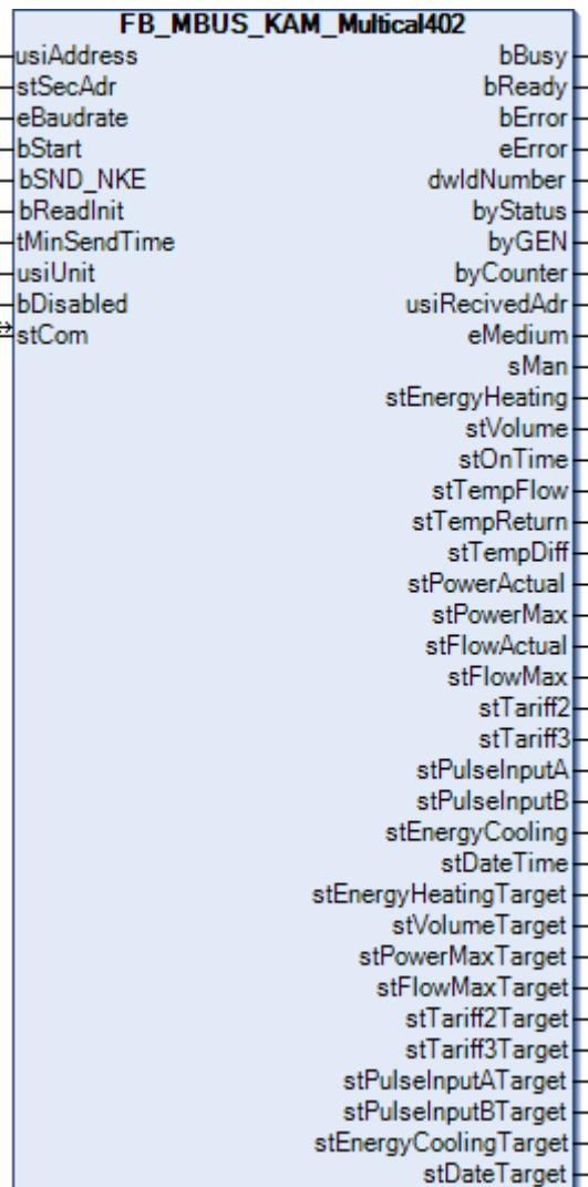
This block is used to read energy meters from Kamstrup.
