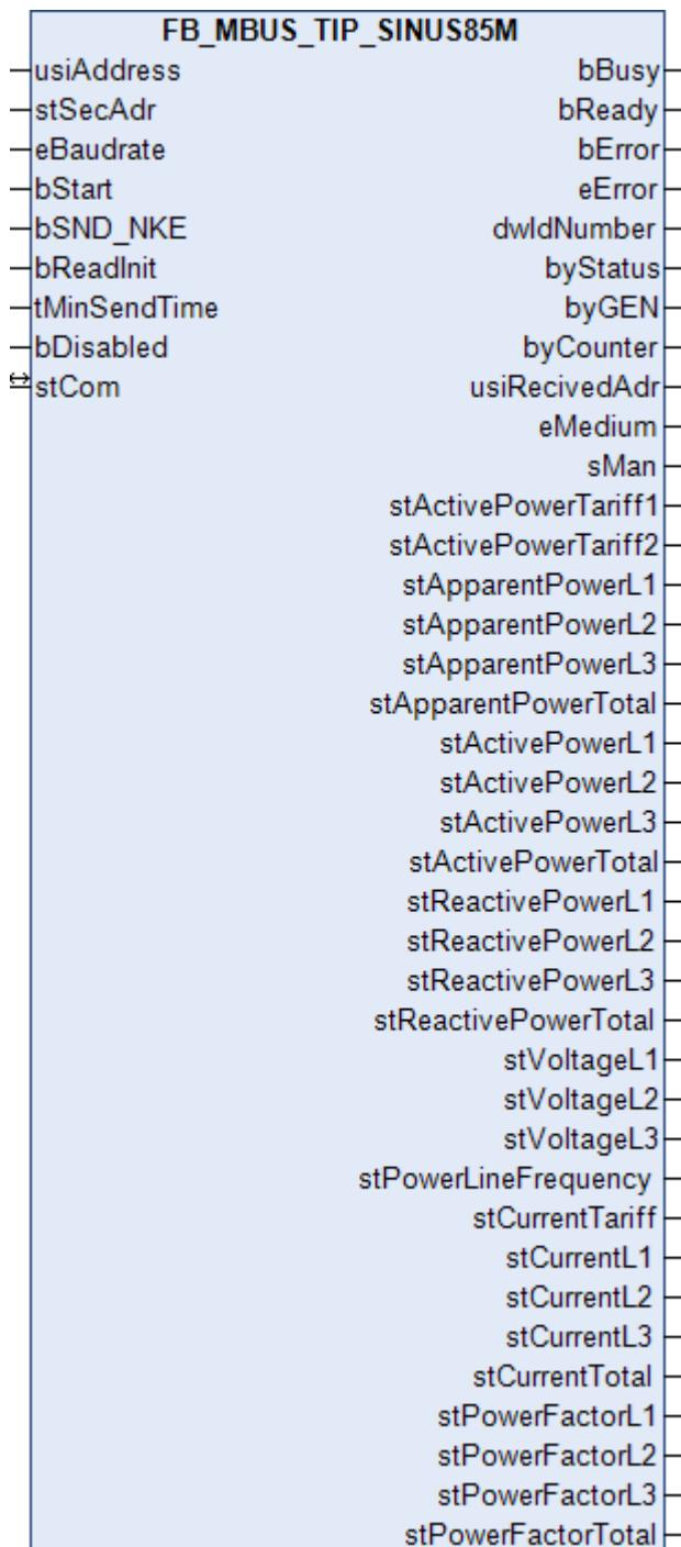
This function block is used to read electricity meters from Thüringer Industrie Produkte GmbH.
