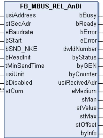
This block is used for reading analog converters from Relay:
