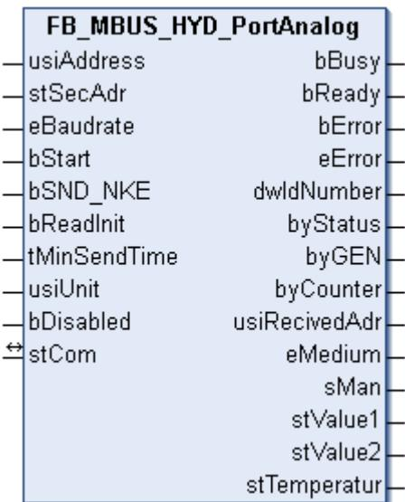
This block is used for reading energy meters with analog output from Hydrometer:
