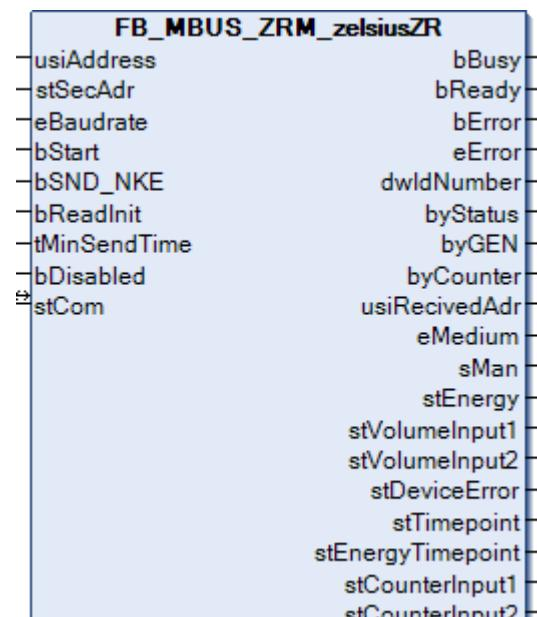
This block is used to read heat meters from Zenner.
