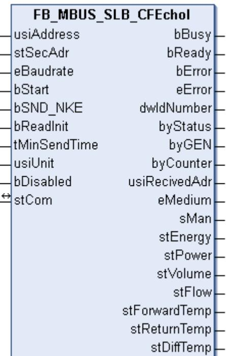
This block is used to read heat meters from Schlumberger:
