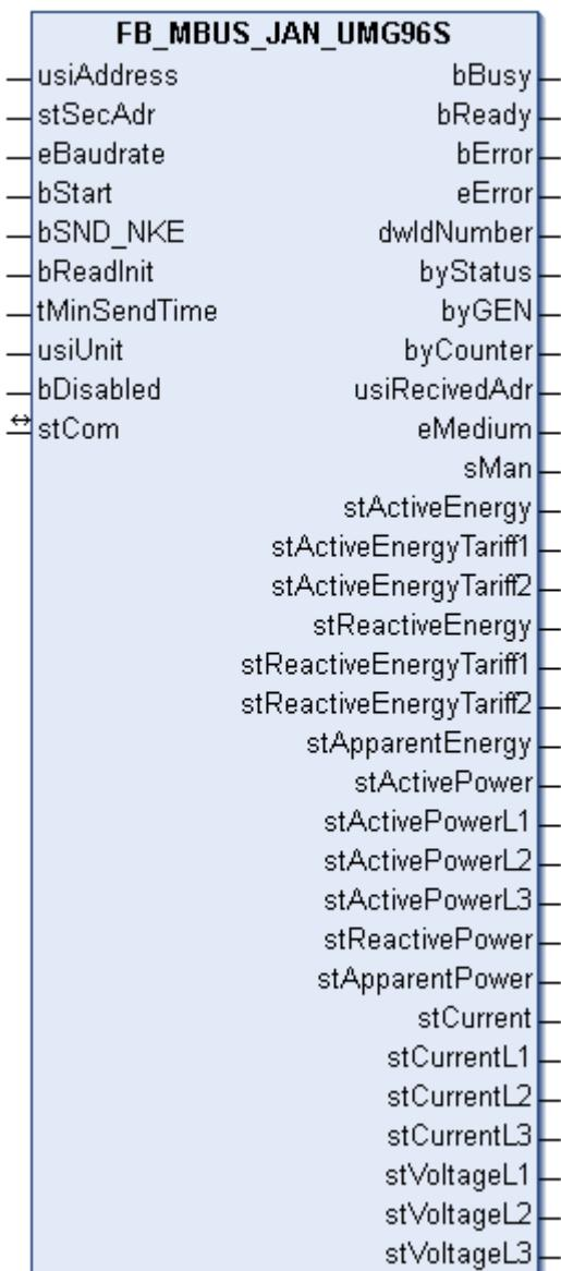
This block is used to read electricity meters from Janitza:
