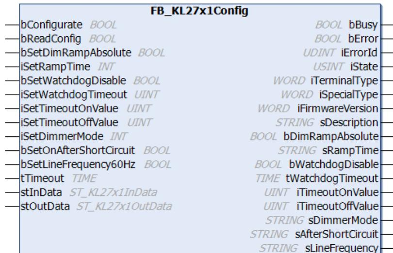
Function block for parameterizing a [KL2751 / KL2761](#): Single-channel dimmer terminal.
