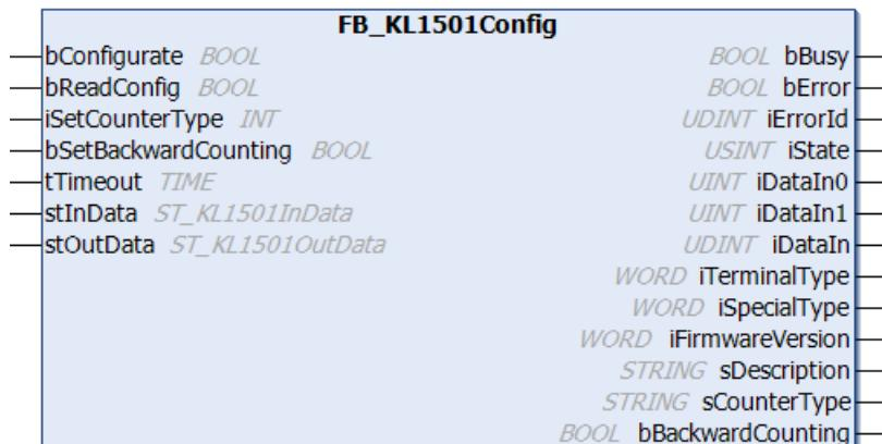
Function block for parameterizing a [KL1501](#): Single-channel counter terminal.
