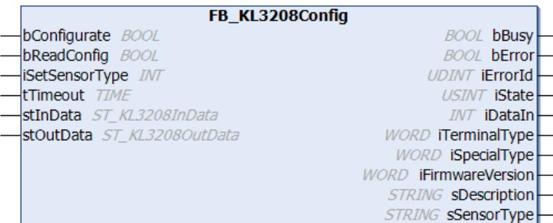
Function block for parameterizing a KL3208-0010: 8-channel input terminal for resistance sensors.
