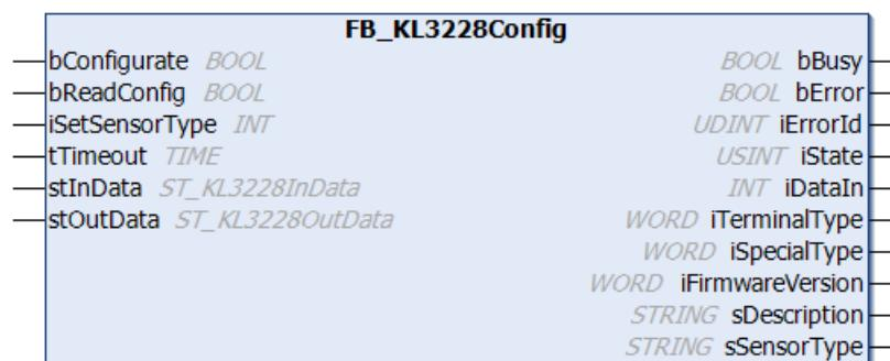
Function block for parameterizing a [KL3228](#): 8-channel input terminal for resistance sensors.
