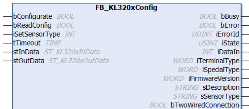
Function block for parameterizing a [KL3201](#), [KL3202](#) or [KL3204](#): Input terminal for resistance sensors.
