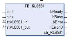
This function block takes care of communication with the KL6581 EnOcean bus terminal. The KL6581 is configured and the data exchange with the EnOcean network is started via this block.
