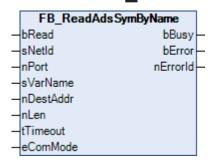
The function block enables reading of any value from another controller using the symbol name.
