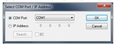
If you want to select a COM port for the firmware update, then select the "COM Port" option. From the drop-down list you can then select "COM1", "COM2", "COM3", "COM4", "COM5", "COM6", "COM7", "COM8", "COM9", "COM10", "COM11", "COM12", "COM13", "COM14", "COM15" or "COM16" as port. The "Search..." button is disabled.
