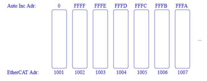
**EtherCAT** Addr: The "EtherCAT Addr" NumericUpDown control contains the address of an EtherCAT slave device. This address is assigned by the EtherCAT master device during the start-up phase. To change the default value, you must first check the checkbox to the left of the NumericUpDown control. If the checkbox to the left of the NumericUpDown control is not checked, the EtherCAT address of the slave device may change if another box is inserted into the communication ring.
