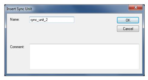
In the "Insert Sync Unit" dialog you can enter a name for the new Sync Unit in the "Name" text box. You can enter a comment in the "Comment" text box. Click "OK" to create the new Sync Unit and close the dialog, click "Cancel" to close the dialog without creating a new Sync Unit.
