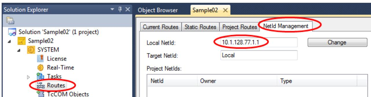
Alternatively, the AMS NetId can be configured locally via the Router category in the TwinCAT SysTray menu. The device must be restarted after changing the AMS NetId.
