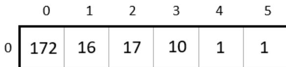
The AMSNetId is purely logical and has usually no relation to the IP address. The AMSNetId is configured at the target system. At the PC for this the TwinCAT System Control is used. If you use other hardware, see the considering documentation for notes about settings of the AMS NetId.
