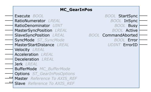
The function block *MC\_GearInPos* synchronizes a slave axis precisely with a master axis (flying saw). The synchronous velocity is achieved exactly at the synchronous point of the master and slave.
