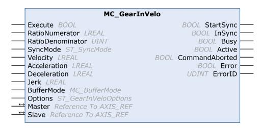
The function block *MC\_GearInVelo* activates a linear master-slave coupling (gear coupling). If the master axis is already moving, the slave axis synchronizes to the master velocity. The function block accepts a fixed gear ratio in numerator/denominator format.
