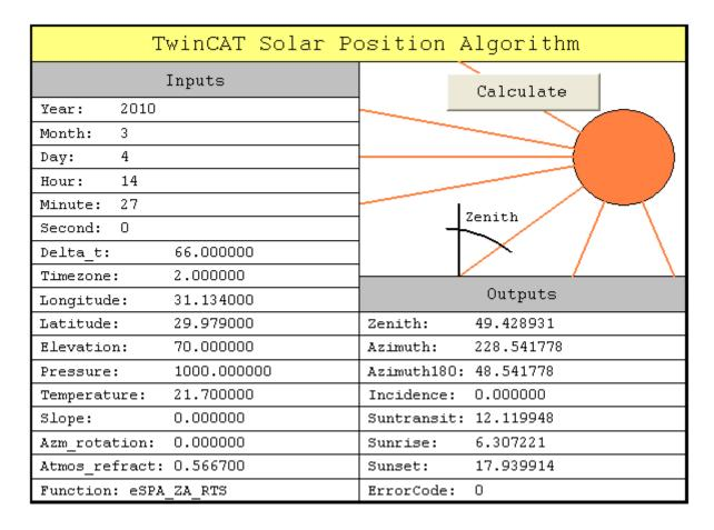
The sun angles at other locations and at other times within the given value ranges can be calculated accordingly. If an input parameter is invalid, an *eErrorCode* with the corresponding enumeration value for the error is displayed.
