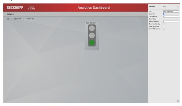
⇒ The changes made are saved client-side (on the device where you open the dashboard) and are only displayed there. In the future, storage will be performed via the HMI server, which means that changes will be made globally on each device.
