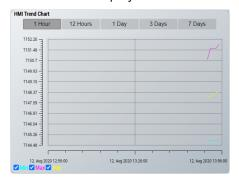
No other HMI controls can be added to the function block, as it is intended exclusively for displaying the Trend Line Control.
