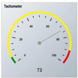
4. The Radial Gauge Control visualizes the input value including the configured limit values.
