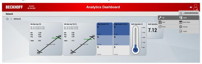
In edit mode, a grid is visible in the background, on which the controls can be arranged as desired.
