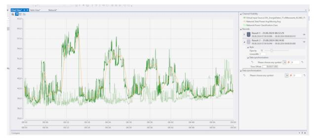
6. If the start times of the data sets do not match, you can adjust them for a direct comparison. This can be done either by manually entering the time offset or by an automatic edge search.
