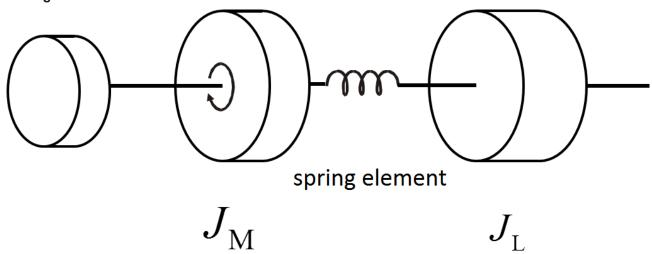
Each coupling between load and motor has a finite rigidity. This leads to different inertia ratios and different resonant frequencies of the complete system. These different frequencies are difficult to determine without a suitable tool. The frequency analysis can be performed with an almost infinitely fine graduation in order to reliably detect all resonance points.
