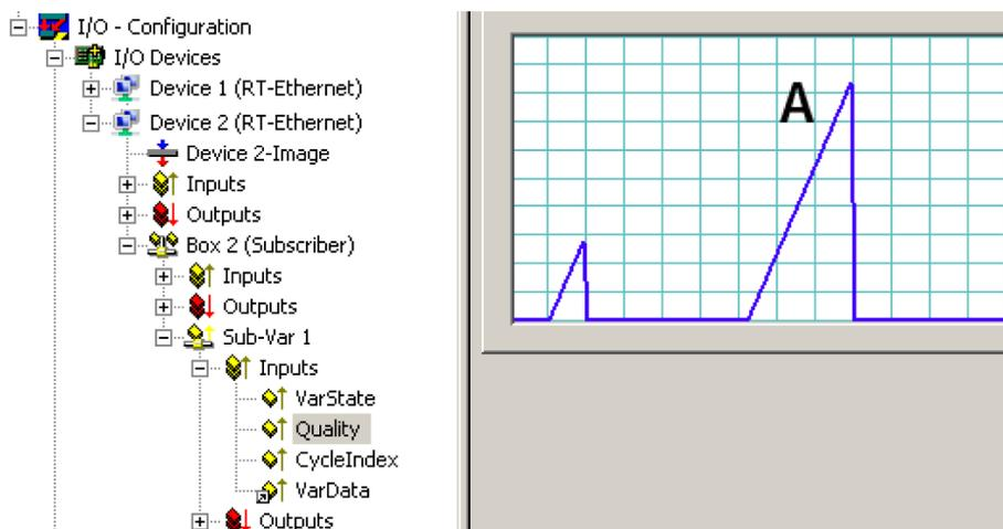
Fig. 2 TwinCAT System Manager with diagnostic function for viewing the latency times of the individual variables.
