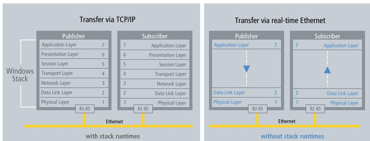
Fig. 3 Realtime-Ethernet: Transfer without stack runtimes, in contrast to TCP/IP
