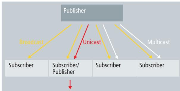
Fig. 1 Broadcast, multicast and unicast as communication modes
