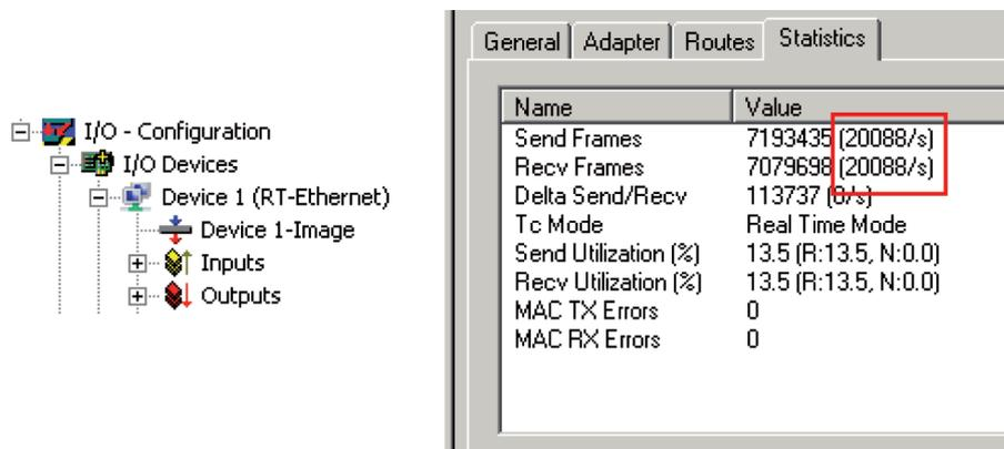
Fig. 8: 50- $\mu$ s inter-PC communication
