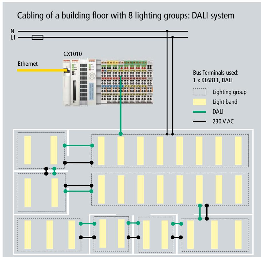
Fig. 11 Simplified cabling with DALI
