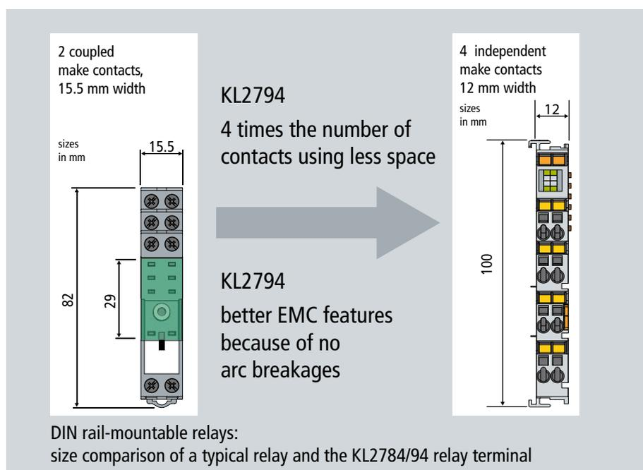
Fig. 4 DIN rail-mountable relays: size comparison of a typical relay and the KL2784/94 relay terminals
