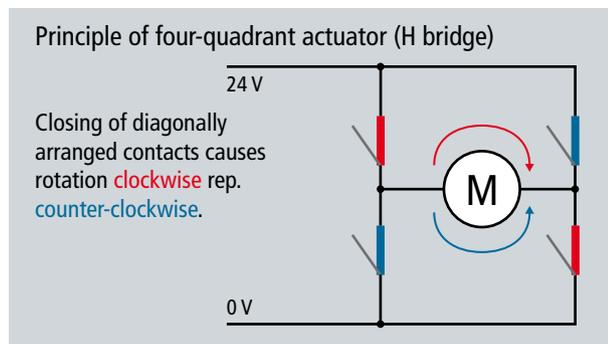
Fig. 3 Four-quadrant actuator
