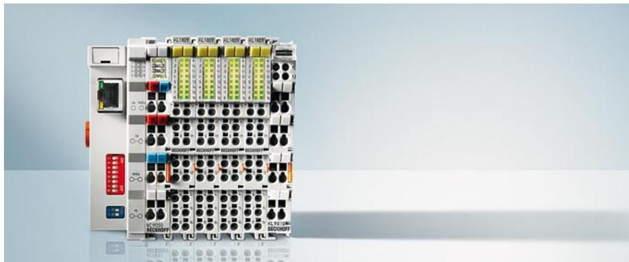
Fig. 1 Exceptionally compact control: Ethernet Controller with integrated IEC 61131-3 PLC functionality combined with 64 digital I/Os including end terminal in a mere 104 mm mounting space.
